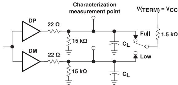
Figure 1. Differential Driver Switching Load
