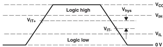
Figure 3. Single-Ended Receiver Input Signal Parameter Definitions
