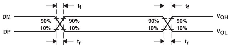
NOTE: The  $t_r/t_f$  ratio is measured as  $t_r(DP)/t_f(DM)$  and  $t_r(DM)/t_f(DP)$  at each crossover point.
