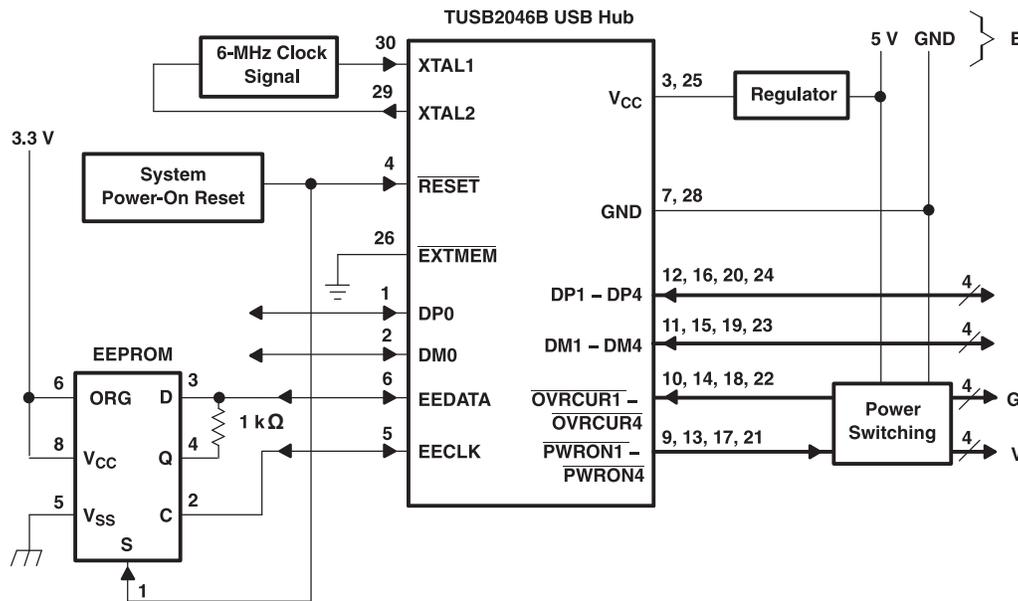
Figure 8. Typical Application of the TUSB2046x USB Hub
