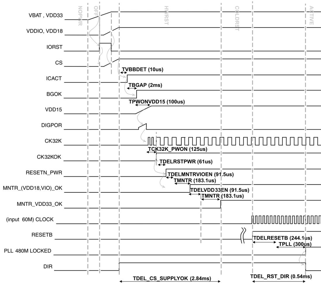
Figure 4-1. TUSB1210 Power-Up Timing (ULPI Clock Input Mode)
