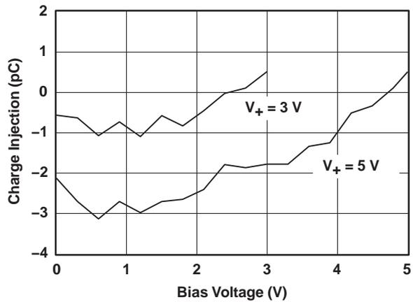
**Figure 5. Charge-Injection ( $Q_C$ ) vs  $V_{COM}$**
