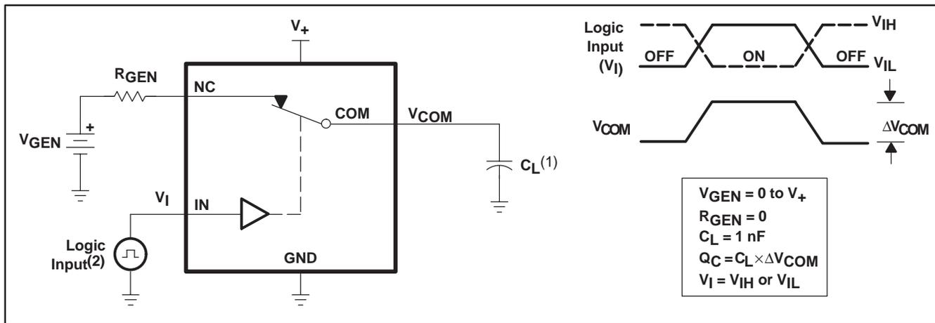
(1)  $C_L$  includes probe and jig capacitance.
