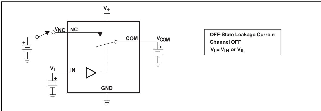
Figure 14. OFF-State Leakage Current ( $I_{COM(OFF)}$ ,  $I_{NC(OFF)}$ )
