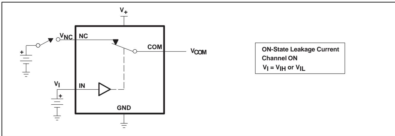
Figure 15. ON-State Leakage Current ( $I_{COM(ON)}$ ,  $I_{NC(ON)}$ )
