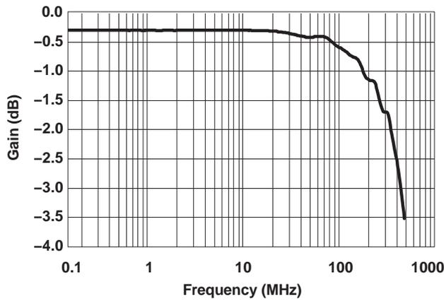
**Figure 9. Bandwidth (Gain vs Frequency) ( $V_+ = 5\text{ V}$ )**
