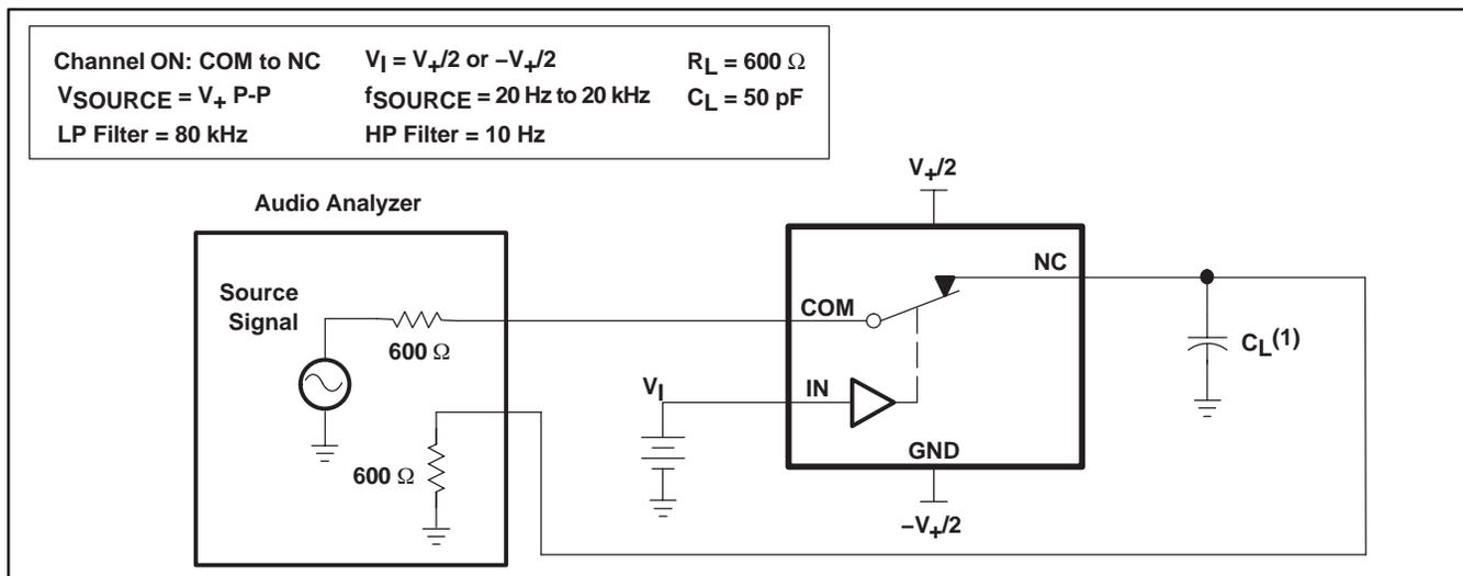
(1)  $C_L$  includes probe and jig capacitance.
