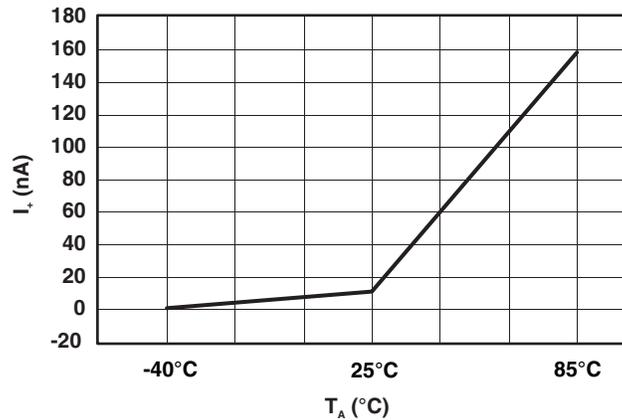
**Figure 14. Power-Supply Current vs Temperature
