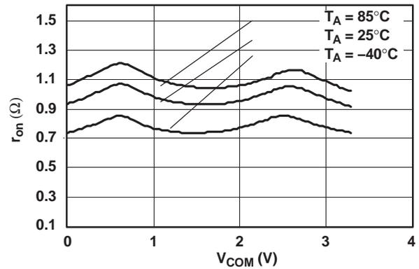
Figure 3.  $r_{on}$  vs  $V_{COM}$  ( $V_+ = 3.3$  V)
