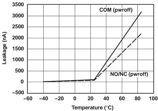
Figure 6. Leakage Current vs Temperature ( $V_+ = 5$  V)
