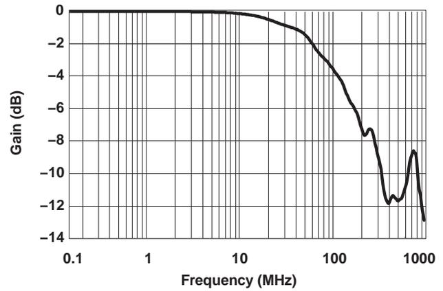
Figure 11. Bandwidth ( $V_+ = 5\text{ V}$ )
