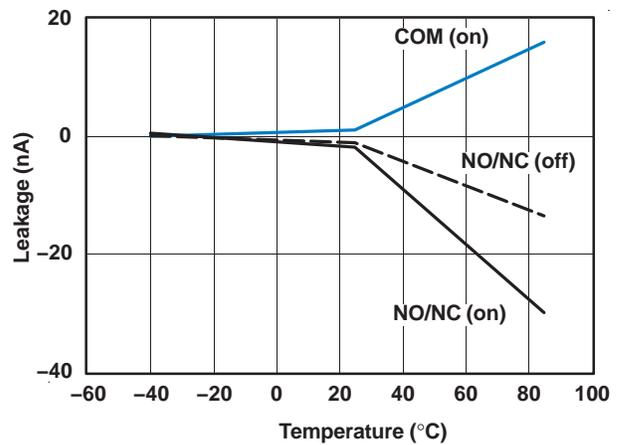
Figure 5. Leakage Current vs Temperature ( $V_+ = 3.3$  V)
