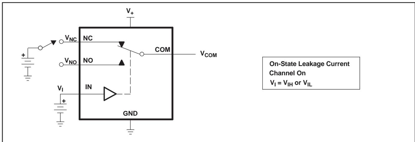
Figure 17. On-State Leakage Current ( $I_{COM(ON)}$ ,  $I_{NC(ON)}$ ,  $I_{NO(ON)}$ )
