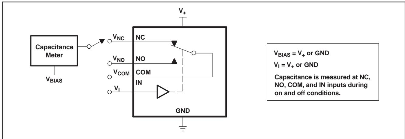
Figure 18. Capacitance ( $C_I$ ,  $C_{COM(ON)}$ ,  $C_{NC(OFF)}$ ,  $C_{NO(OFF)}$ ,  $C_{NC(ON)}$ ,  $C_{NO(ON)}$ )
