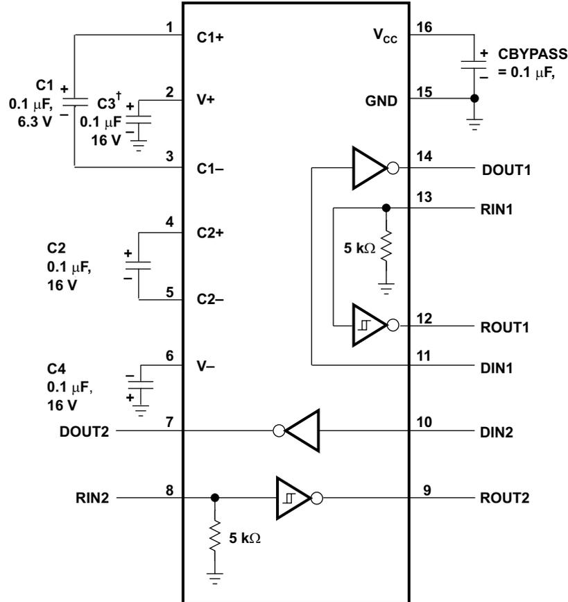
† C3 can be connected to  $V_{CC}$  or GND.
