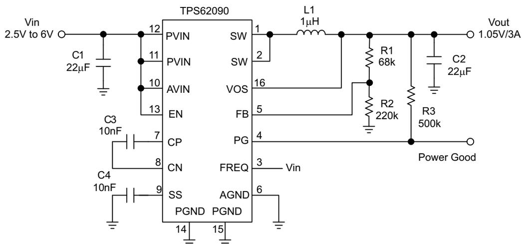
Figure 32. 1.05 V Adjustable Version Operating at 1.4 MHz
