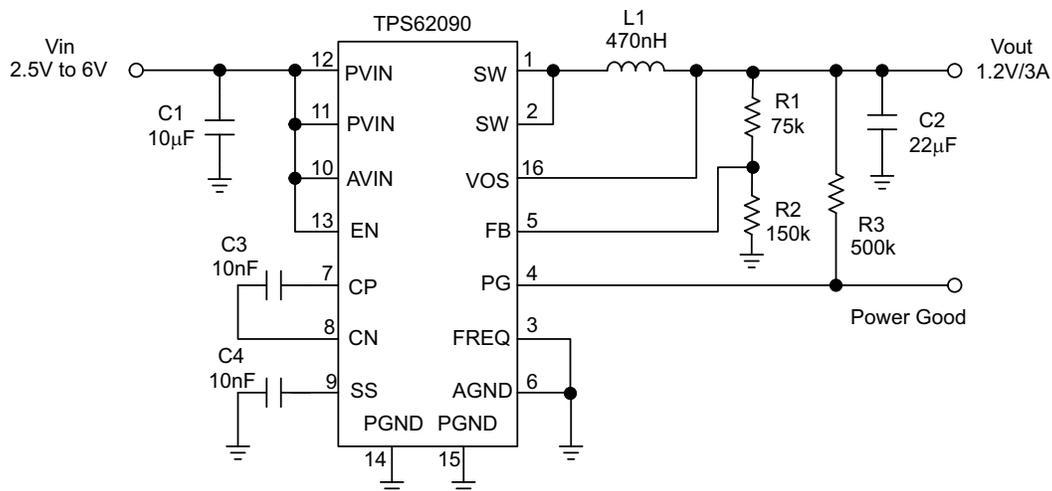
Figure 29. 1.2 V Adjustable Version Operating at 2.8 MHz
