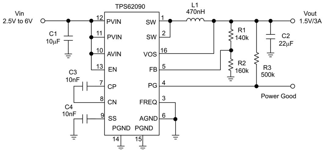
Figure 30. 1.5 V Adjustable Version Operating at 2.8 MHz
