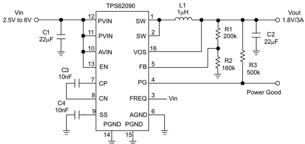
Figure 31. 1.8 V Adjustable Version Operating at 1.4 MHz
