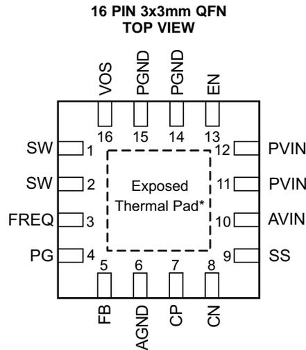
NOTE: \*The exposed Thermal Pad is connected to AGND.
