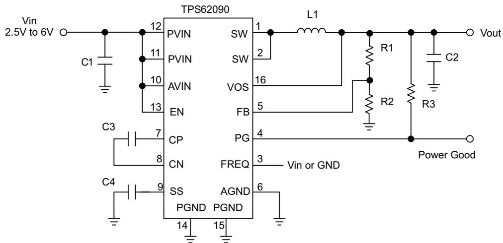
**Figure 1. Parametric Measurement Circuit**
