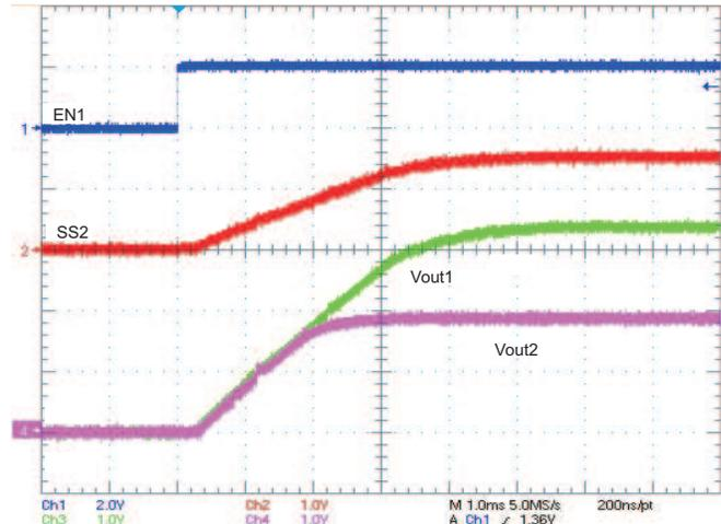
Figure 23. Ratio-metric Start-Up using Coupled SS/TR Pins
