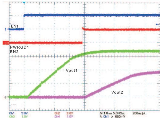
Figure 19. Sequential Startup using EN and PWRGD
