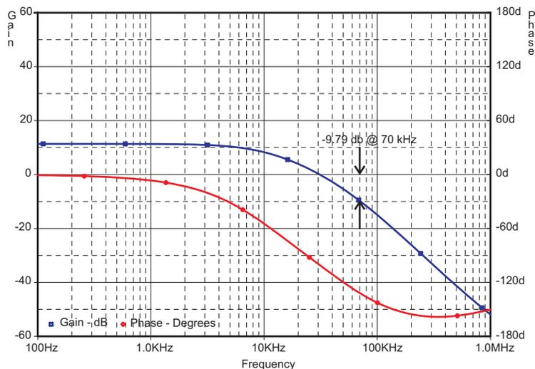
**Figure 28. Power Stage Gain and Phase Characteristics**
