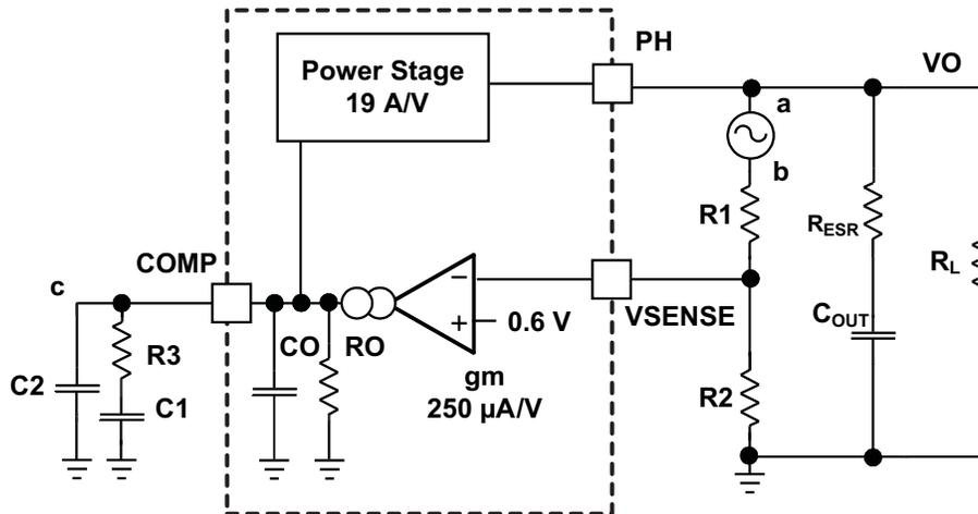
Figure 24. Small Signal Model for Loop Response
