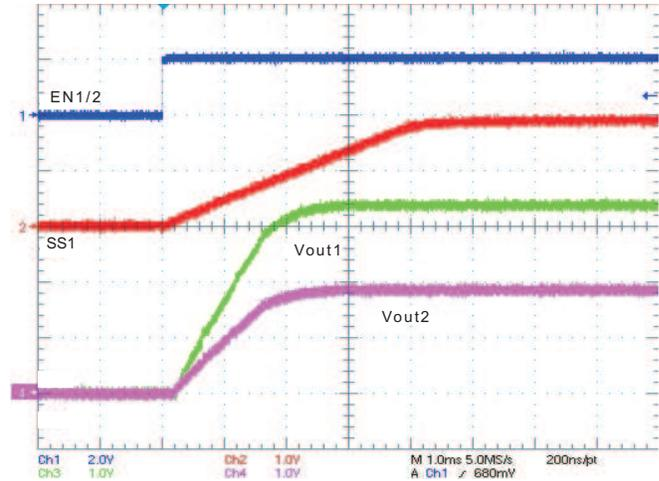
Figure 21. Ratio-metric Startup with Vout1 Leading Vout2
