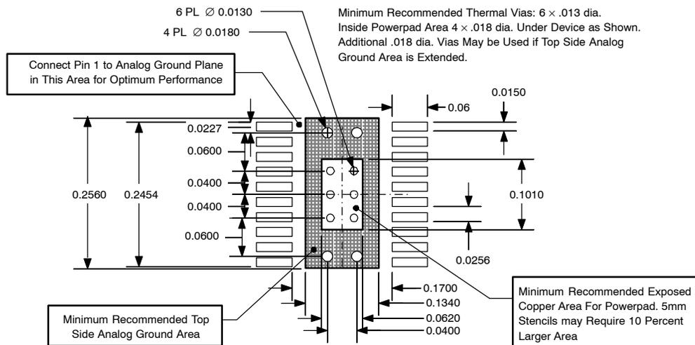
**Figure 12. Recommended Land Pattern for 20-Pin PWP PowerPAD**
