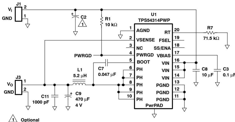
Figure 10. TPS54314 Schematic
