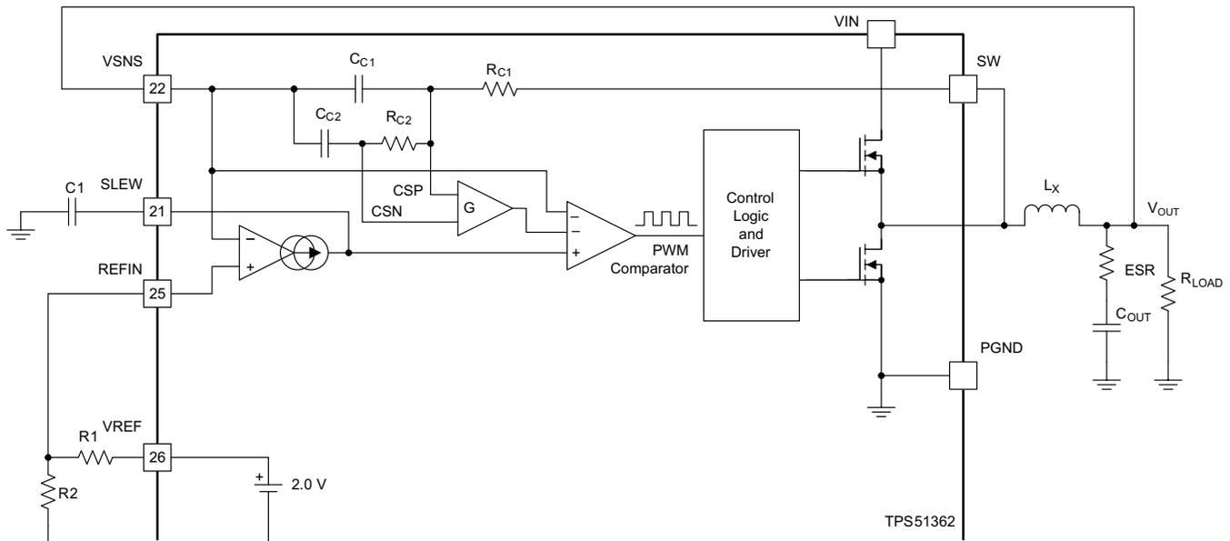
**Figure 21. Simplified Architecture Illustrating DCAP2 Mode**
