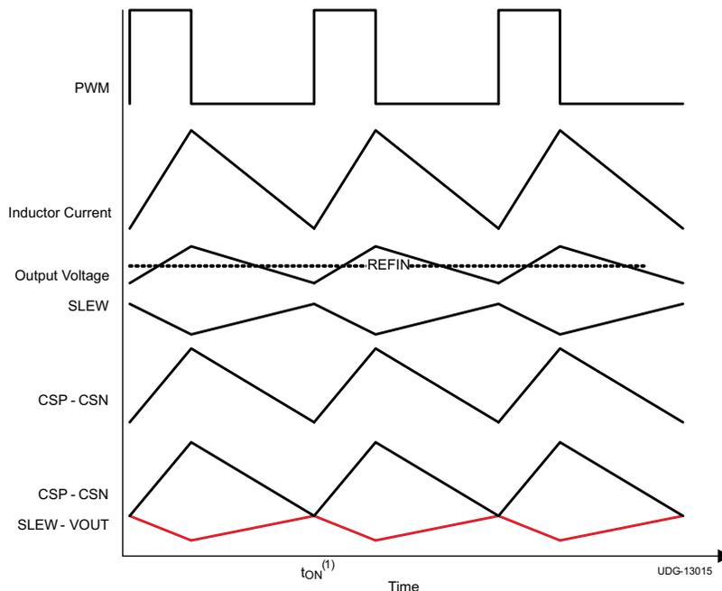
**Figure 20. On-Time Waveforms** <sup>(1)</sup>
