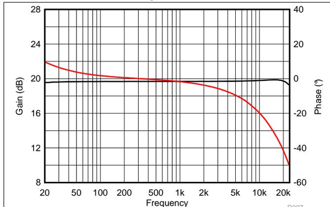
AVCC=PVCC = 12 V, Load = 6  $\Omega$  + 47  $\mu\text{H}$  (device pins)
