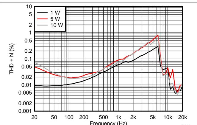
AVCC=PVCC = 13 V, Load = 4  $\Omega$  + 33  $\mu\text{H}$ , 1 W, 2.5 W, 10 W
