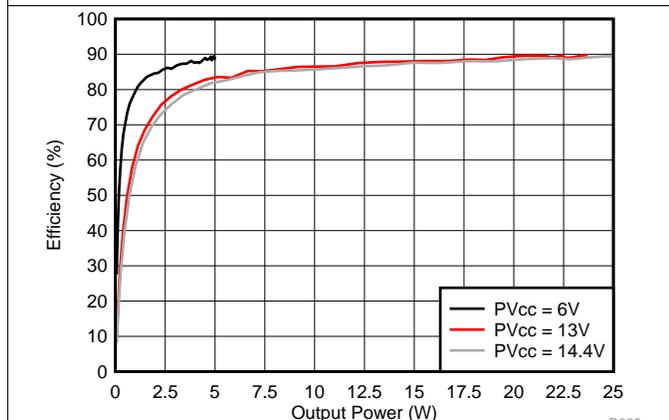
AVCC=PVCC= 6 V, 13 V, 14.4 V, Load = 8  $\Omega$  + 66  $\mu\text{H}$ , AGL + PLIM disable (LIMRATE = GND, LIMTHRES = GVDD)
