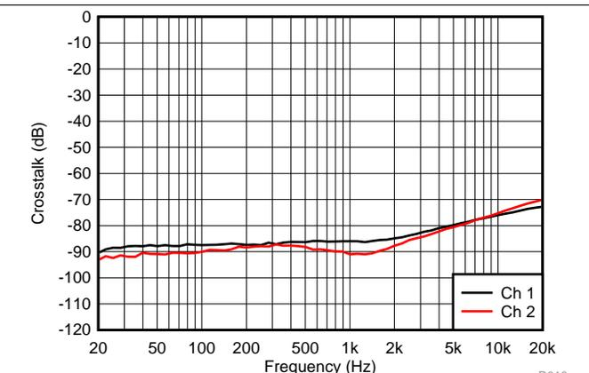
AVCC=PVCC = 12 V, 1 W, Load = 6  $\Omega$  + 47  $\mu\text{H}$
