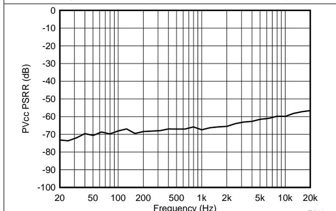
AVCC=PVCC = 12 V, Load = 4  $\Omega$  + 33  $\mu\text{H}$
