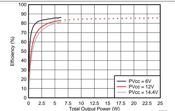
AVCC=PVCC = 6 V, 12 V, 14.4 V, Load = 6  $\Omega$  + 47  $\mu\text{H}$ , AGL + PLIM disable (LIMRATE = GND, LIMTHRES = GVDD)
