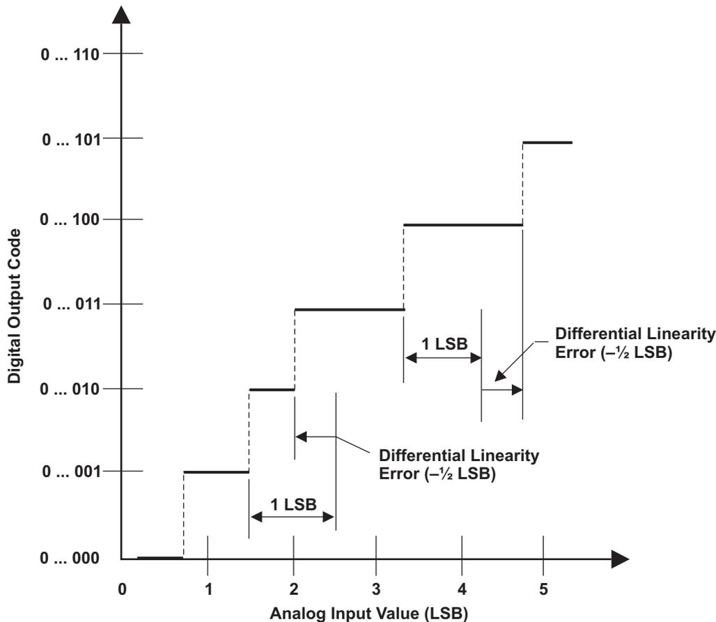
NOTE A:  $1 \text{ LSB} = (AD_{\text{REFHI}} - AD_{\text{REFLO}}) / 2^n$  where  $n=10$  in 10-bit mode and 12 in 12-bit mode
