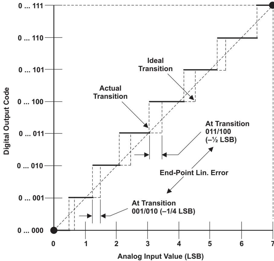
NOTE A:  $1 \text{ LSB} = (AD_{\text{REFHI}} - AD_{\text{REFLO}}) / 2^n$  where  $n=10$  in 10-bit mode and 12 in 12-bit mode
