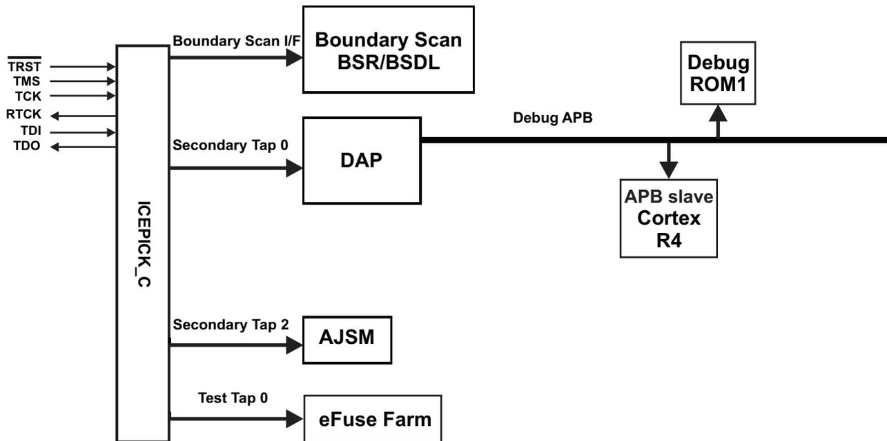
Figure 6-14. Debug Subsystem Block Diagram
