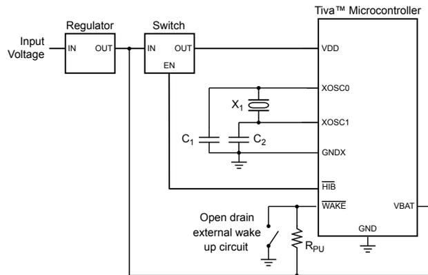
**Note:** Some devices may not supply a  $GNDX$  signal. See “Signal Tables” on page 1354 for pins specific to your device.
