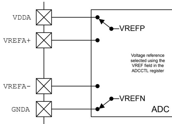
The range of this conversion value is from 0x000 to 0xFFFF. In single-ended-input mode, the 0x000 value corresponds to the voltage level on VREFN; the 0xFFFF value corresponds to the voltage level on VREFP. This configuration results in a resolution that can be calculated using the following equation:
