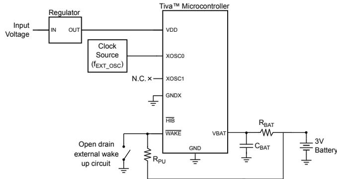
**Note:** Some devices may not supply the GNDX,  $\overline{WAKE}$  or  $\overline{HIB}$  signals. See “Signal Tables” on page 1354 for pins specific to your device.
