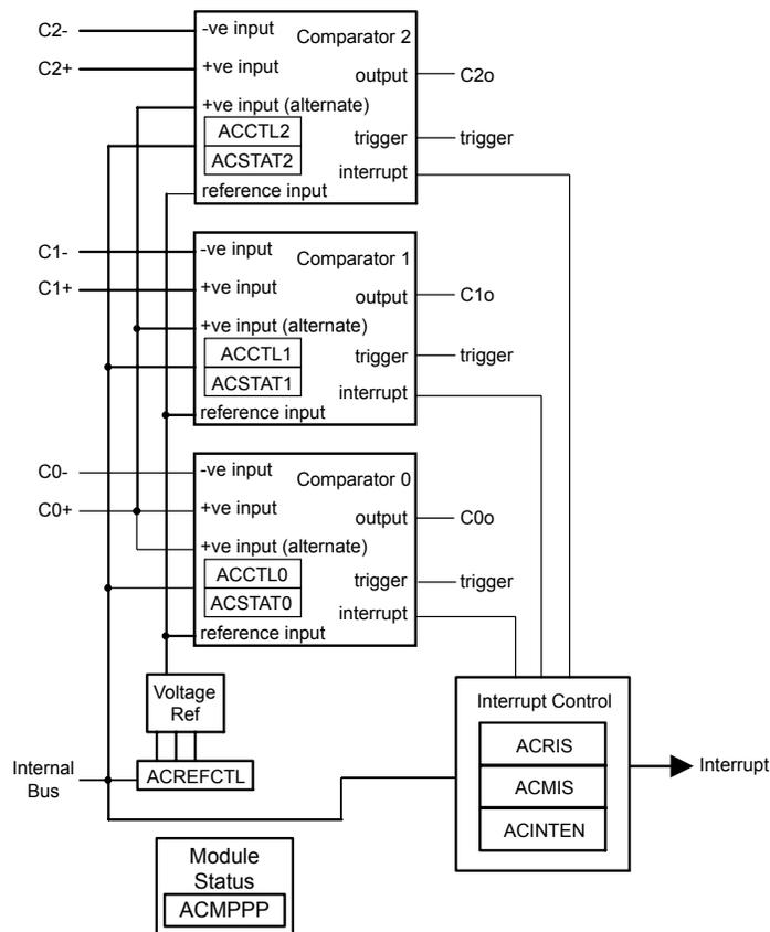
**Note:** This block diagram depicts the maximum number of analog comparators and comparator outputs for the family of microcontrollers; the number for this specific device may vary. See page 1250 for what is included on this device.
