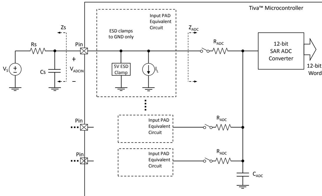
The ADC operates from both the 3.3-V analog and 1.2-V digital power supplies. The ADC clock can be configured to reduce power consumption when ADC conversions are not required (see “System Control” on page 227). The analog inputs are connected to the ADC through specially balanced input paths to minimize the distortion and cross-talk on the inputs. Detailed information on the ADC power supplies and analog inputs can be found in “Analog-to-Digital Converter (ADC)” on page 1426.
