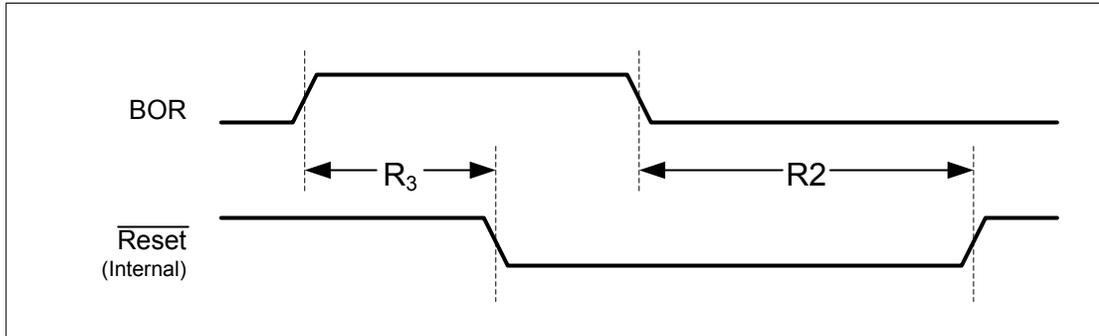
Figure 24-11. External Reset Timing ( $\overline{RST}$ )
