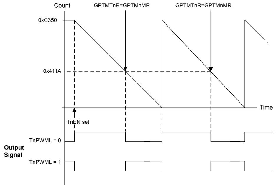
When synchronizing the timers using the **GPTMSYNC** register, the timer must be properly configured to avoid glitches on the CCP outputs. Both the  $TnPLO$  and the  $TnMRSU$  bits must be set in the **GPTMTnMR** register. Figure 11-6 on page 731 shows how the CCP output operates when the  $TnPLO$  and  $TnMRSU$  bits are set and the **GPTMTnMATCHR** value is greater than the **GPTMTnILR** value.
