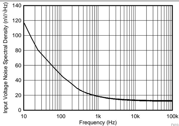
Figure 9. Input Voltage Noise Spectral Density vs Frequency
