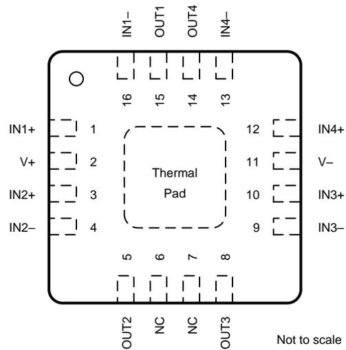
Connect thermal pad to V-.
