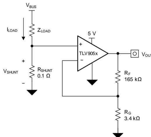
Figure 41. TLV905x in a Low-Side, Current-Sensing Application
