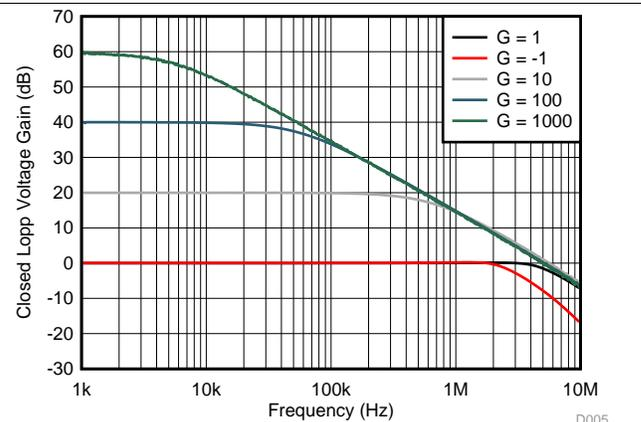
Figure 16. Closed Loop Voltage Gain vs Frequency
