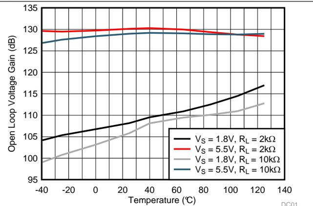
Figure 14. Open Loop Voltage Gain vs Temperature
