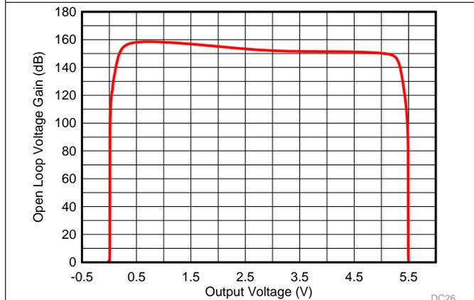
Figure 15. Open Loop Voltage Gain vs Output Voltage
