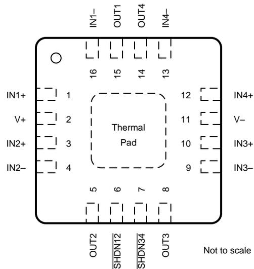
Connect thermal pad to V–.
