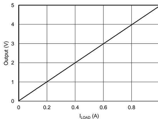
**Figure 42. Low-Side, Current-Sense Transfer Function**
