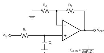
$$\frac{V_{\text{OUT}}}{V_{\text{IN}}} = \left(1 + \frac{R_F}{R_G}\right) \left(\frac{1}{1 + sR_1 C_1}\right)$$
