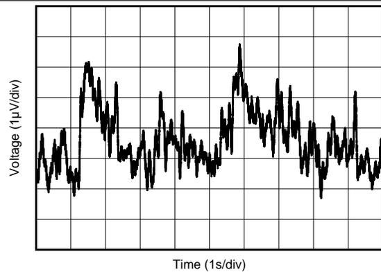
Figure 8. 0.1-Hz to 10-Hz Input Voltage Noise
