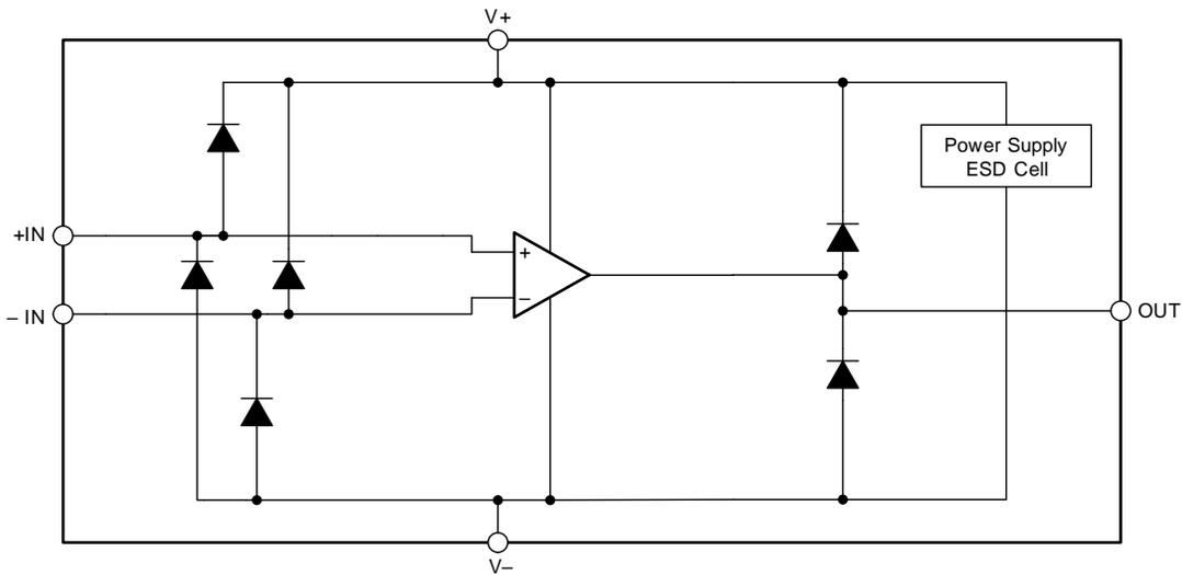
Figure 39. Equivalent Internal ESD Circuitry
