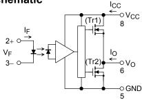
A 0.1  $\mu F$  bypass capacitor must be connected between pin 8 and 5.
