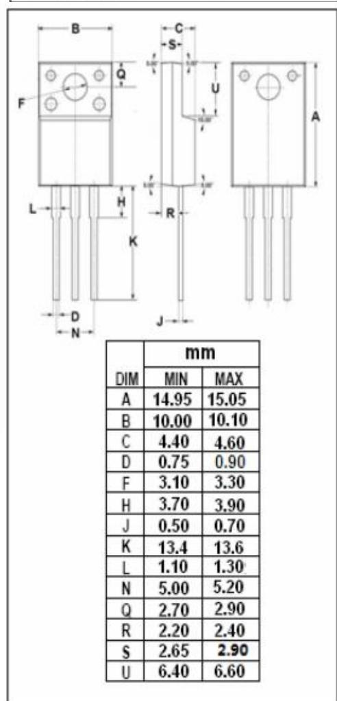
**iscN-Channel MOSFET Transistor****TK16A60W, ITK16A60W****ELECTRICAL CHARACTERISTICS** $T_c=25^\circ\text{C}$  unless otherwise specified
