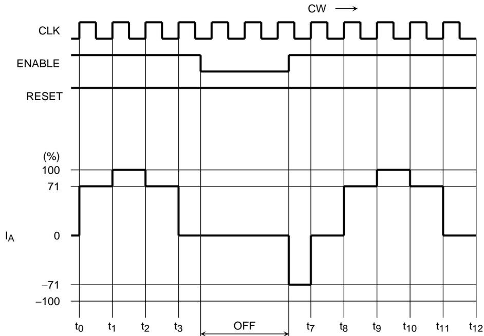
The ENABLE signal at Low level disables only the output signals. Internal logic functions proceed in accordance with input clock signals and without regard to the ENABLE signal. Therefore output current is initiated by the timing of the internal logic circuit after release of disable mode.
