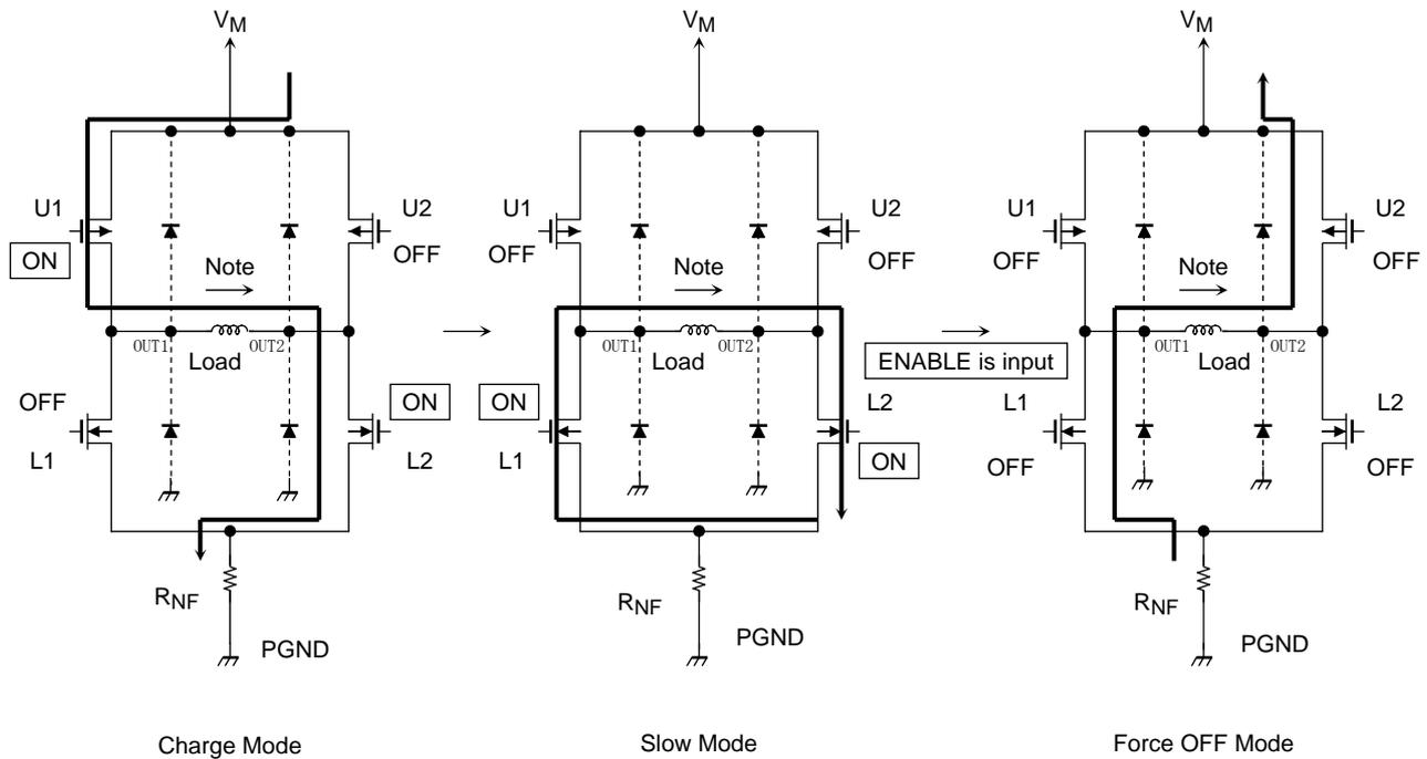
As shown in the figure above, an output transistor has parasitic diodes. Normally, when the energy of the coil is drawn out, each transistor is turned ON and the power flows in the opposite-to-normal direction; as a result, the parasitic diode is not used. However, when all the output transistors are forced OFF, the coil energy is drawn out via the parasitic diode.
