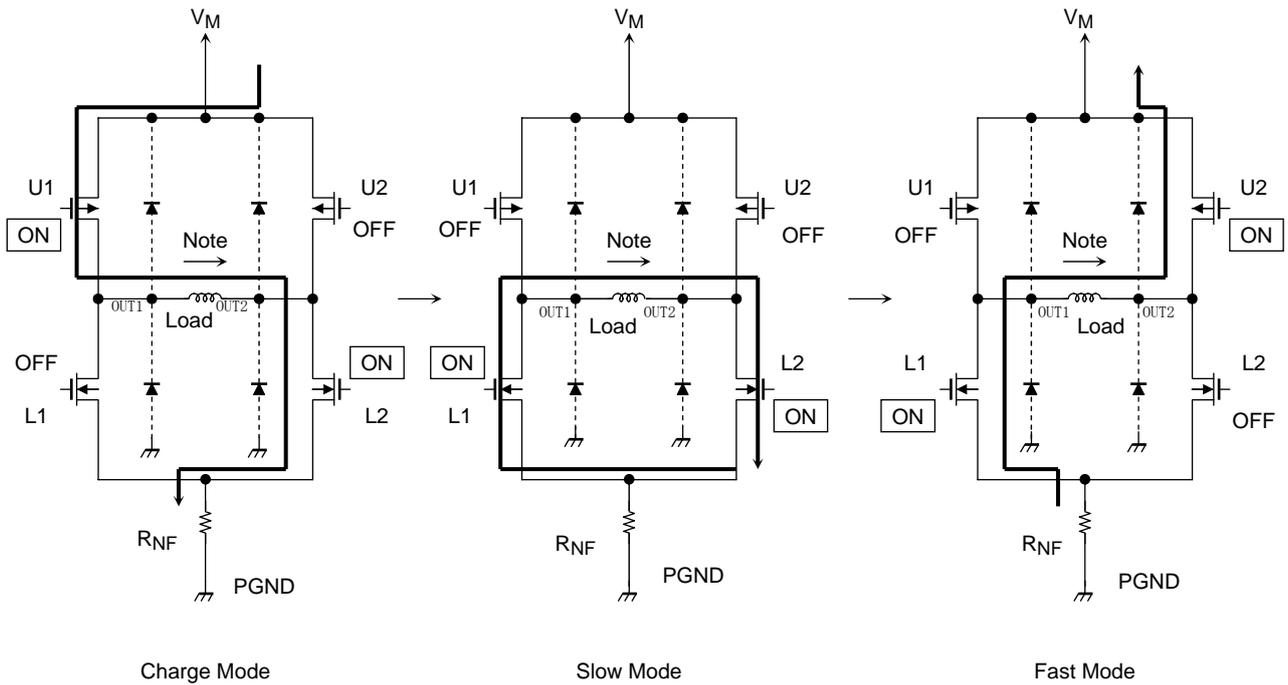
**Output Stage Transistor Operation Functions**
