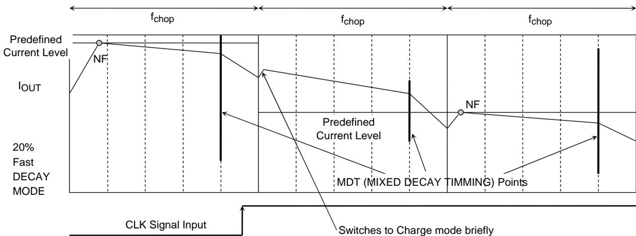
\*: Even if the output current rises above the predefined current at the RNF point, the current control mode is briefly switched to Charge mode for current sensing.
