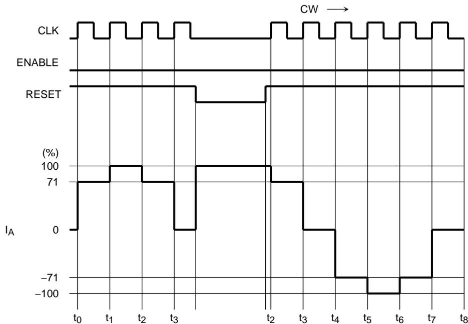
When the RESET signal goes Low level, output goes Initial state (Initial state: A Channel output current is 100%).
