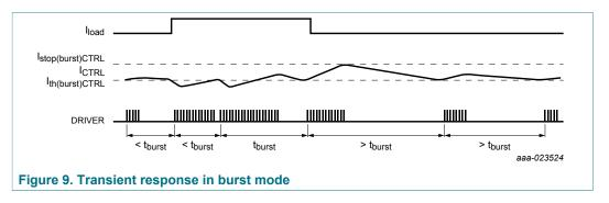
Even though the burst-mode regulates towards a target repetition frequency, the actual repetition rate is lower than the target because of the discrete number of switching cycles. Increasing or decreasing the number of pulses results in a step change in the burst repetition frequency.
