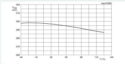
Figure 16. Overpower protection voltage (at  $I_{AUX}$  = 1.46 mA) as a function of temperature
