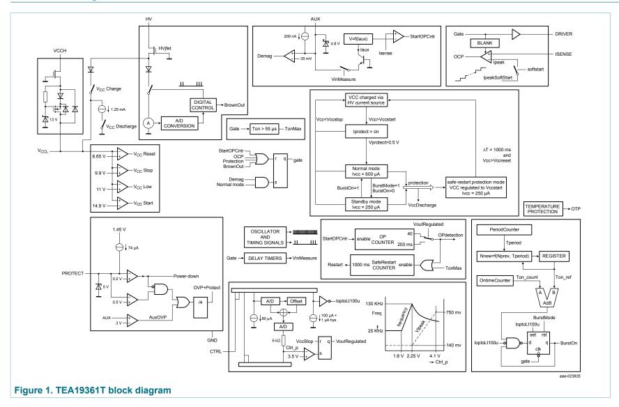
GreenChip SMPS primary side control IC with QR/DCM operation
