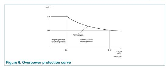
During system start-up, the maximum time-out period is lowered to 40 ms. When the output voltage is within its regulation level, the maximum time-out period returns to 200 ms, limiting the output power to a minimum at a shorted output. Shortening the overpower timer ensures that the input power of the system is limited to < 5 W at a shorted output.
