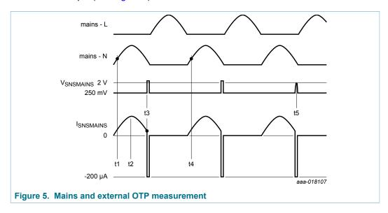
At t1, the voltage at the SNSMAINS pin is internally regulated to  $V_{\text{regd(SNSMAINS)}}$  (250 mV). The current into the SNSMAINS pin is a measure of the system input mains voltage. The TEA19162T continuously measures the SNSMAINS current and waits until it detects a peak in the measured current (t2). This peak current value is internally stored and used as an input for the brownout/brownin detection and the mains compensation.
