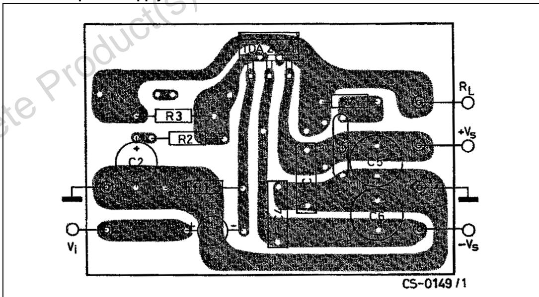
Figure 15. Amplifier with single power supply
