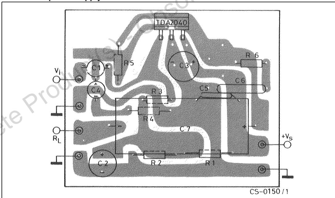
Figure 17. 30-watt bridge amplifier with split power supply
