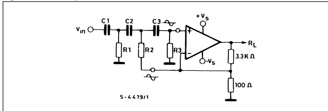
A more effective solution, named "Active Power Filter" by STMicroelectronics, is shown in [Figure 23](#). The proposed circuit can be realized by combined power amplifiers and 12-dB/octave or 18-dB/octave high-pass or low-pass filters.
