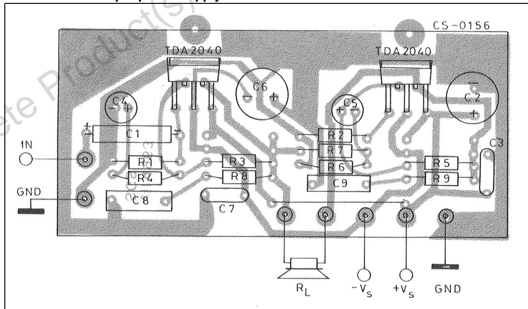
Figure 19. Two-way hi-fi system with active crossover
