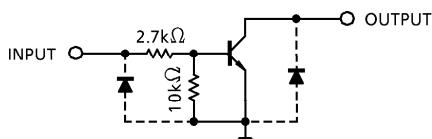
(Note) The input and output parasitic diodes cannot be used as clamp diodes.
