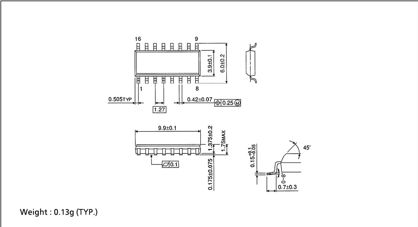
**SSOP 16PIN OUTLINE DRAWING (SSOP16-P-225-0.65B)**
