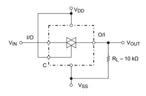
$$R_{ON} = 10 \times \frac{\left(V_{IN} - V_{OUT}\right)}{V_{OUT}} \left[k\Omega\right]$$
