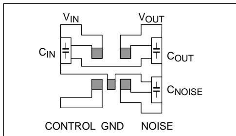
Circuit board material: glass epoxy, Circuit board dimension: 30 mm × 30 mm,
