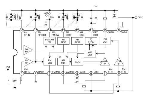
Explanation Of Terminals Terminal voltage: Typical DC voltage at Ta =  $25^{\circ}$ C,  $V_{CC}$  = 3V and no signal with test circuit 1
