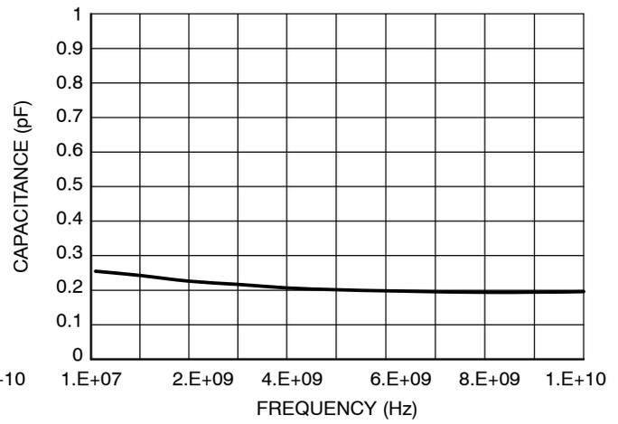
**Figure 4. Typical Capacitance over Frequency
