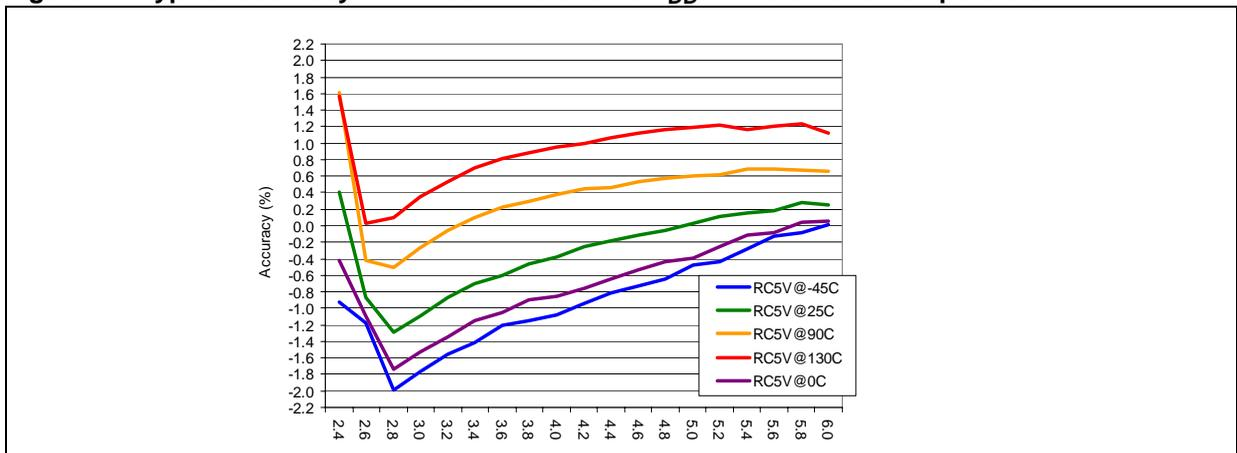
Figure 45. Typical accuracy with RCCR=RCCR1 vs  $V_{DD}$ = 2.4-6.0V and Temperature
