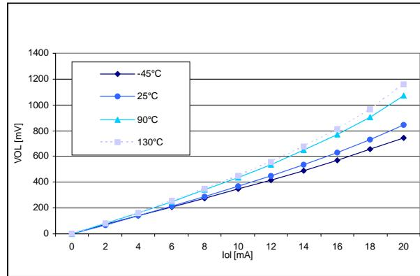
Figure 57. Typical  $V_{OL}$  at  $V_{DD} = 5V$  (standard pins)
