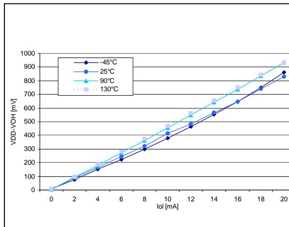
Figure 62. Typical  $V_{DD}-V_{OH}$  at  $V_{DD} = 3V$  (HS pins)
