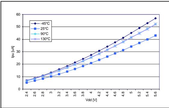
Figure 54. Typical  $R_{PU}$  vs.  $V_{DD}$  with  $V_{IN}=V_{SS}$
