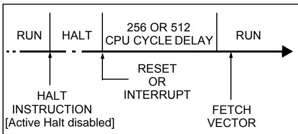
**Figure 28. HALT Mode Flow-chart**
