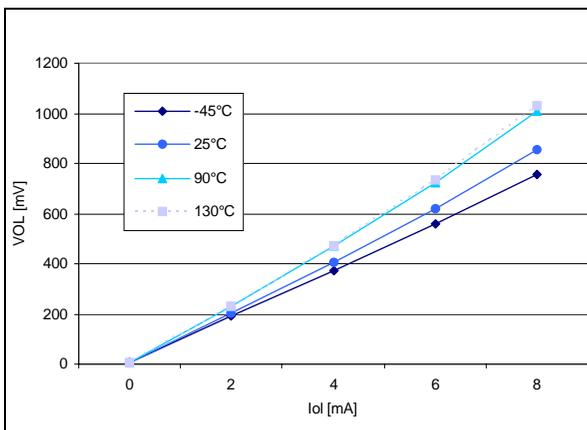
Figure 60. Typical  $V_{OL}$  at  $V_{DD} = 5V$  (HS pins)
