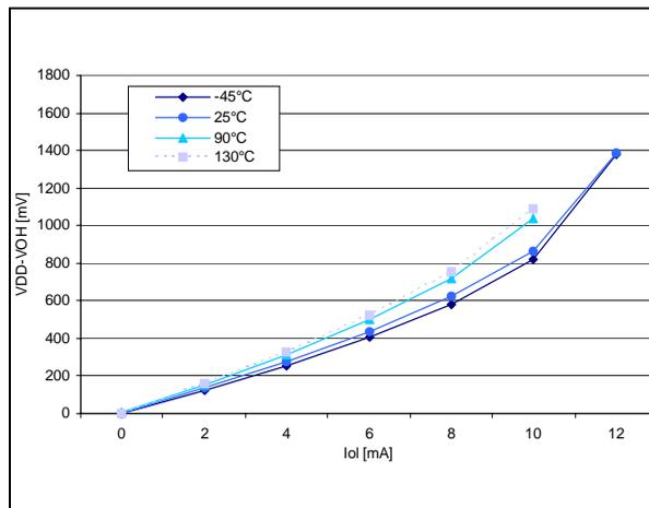
Figure 63. Typical  $V_{DD}-V_{OH}$  at  $V_{DD} = 5V$  (HS pins)
