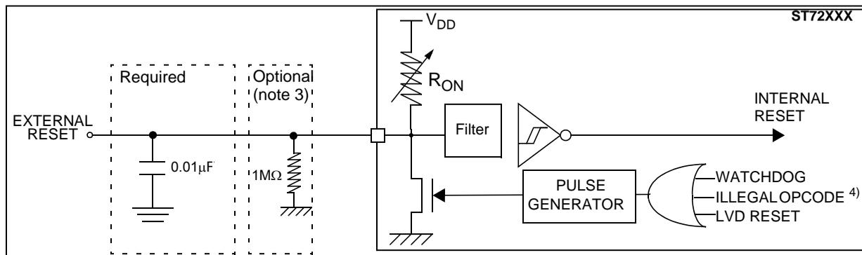
Figure 67.  $\overline{\text{RESET}}$  pin protection when LVD is disabled.<sup>1)</sup>
