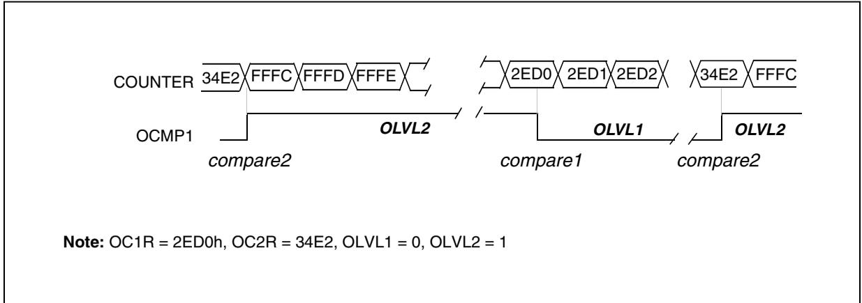
**Note:** On timers with only one Output Compare register, a fixed frequency PWM signal can be generated using the output compare and the counter overflow to define the pulse length.
