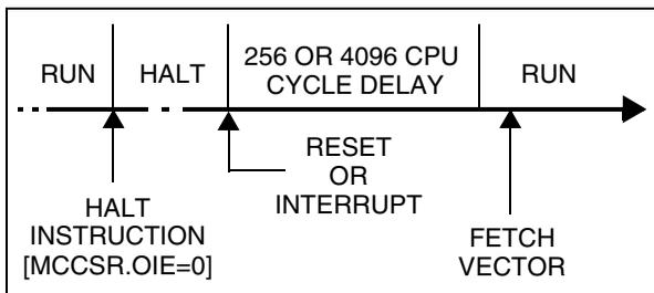
Figure 26. HALT Mode Flow-chart
