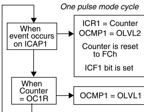
Then, on a valid event on the ICAP1 pin, the counter is initialized to FCh and OLVL2 bit is loaded on the OCMP1 pin, the ICF1 bit is set and the value FFFDh is loaded in the IC1R register.
