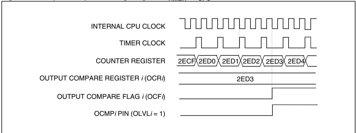
Figure 56. Output Compare Timing Diagram,  $f_{\text{TIMER}} = f_{\text{CPU}}/4$
