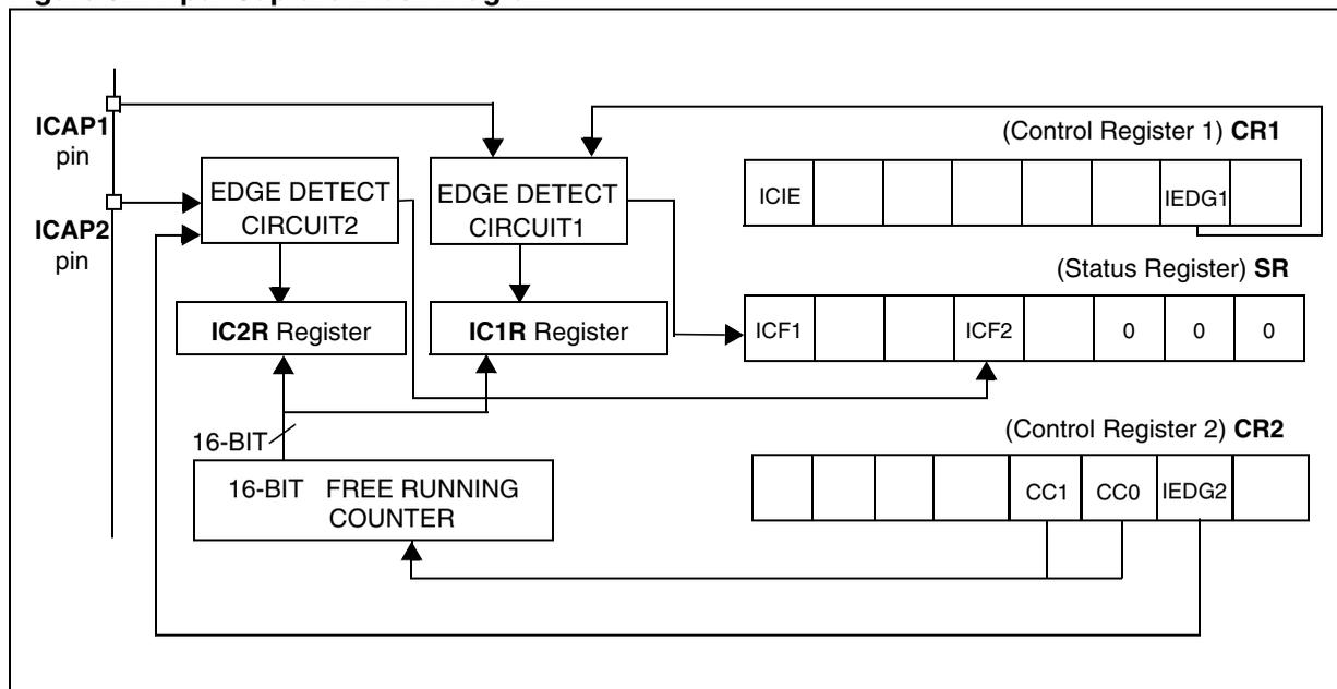
Figure 53. Input Capture Timing Diagram
