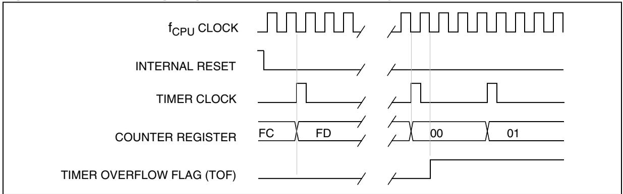
Figure 62. Counter Timing Diagram, Internal Clock Divided by 8
