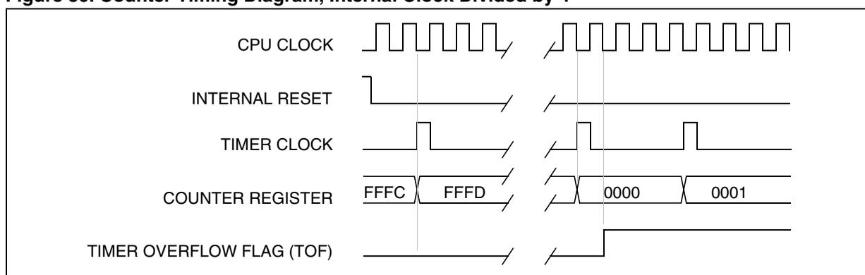
Figure 51. Counter Timing Diagram, Internal Clock Divided By 8
