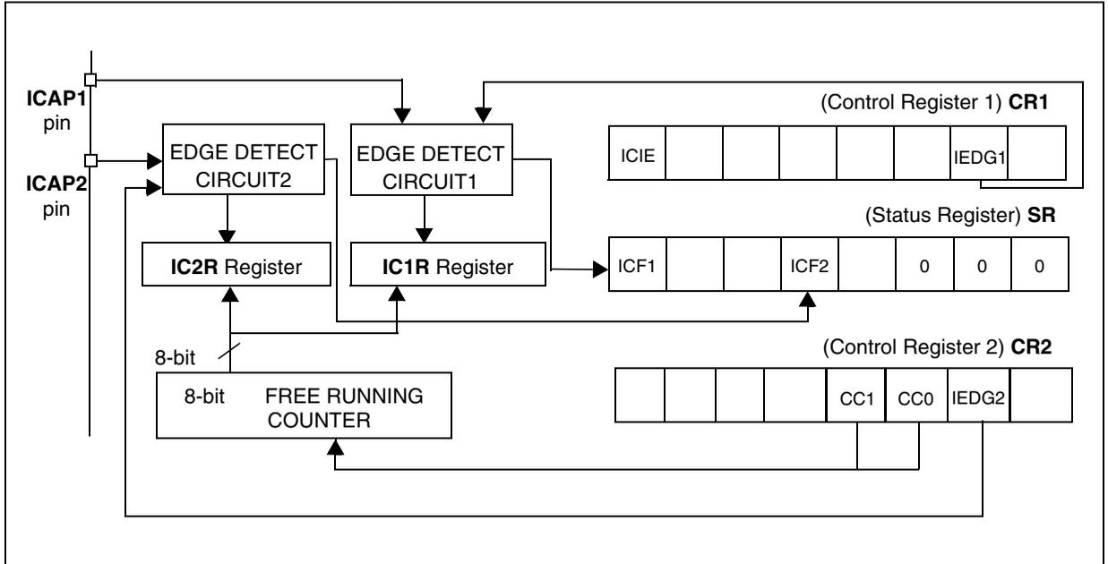
Figure 64. Input Capture Timing Diagram
