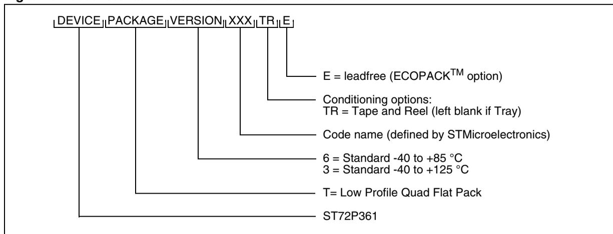
Figure 131. FASTROM Factory Coded Device Types
