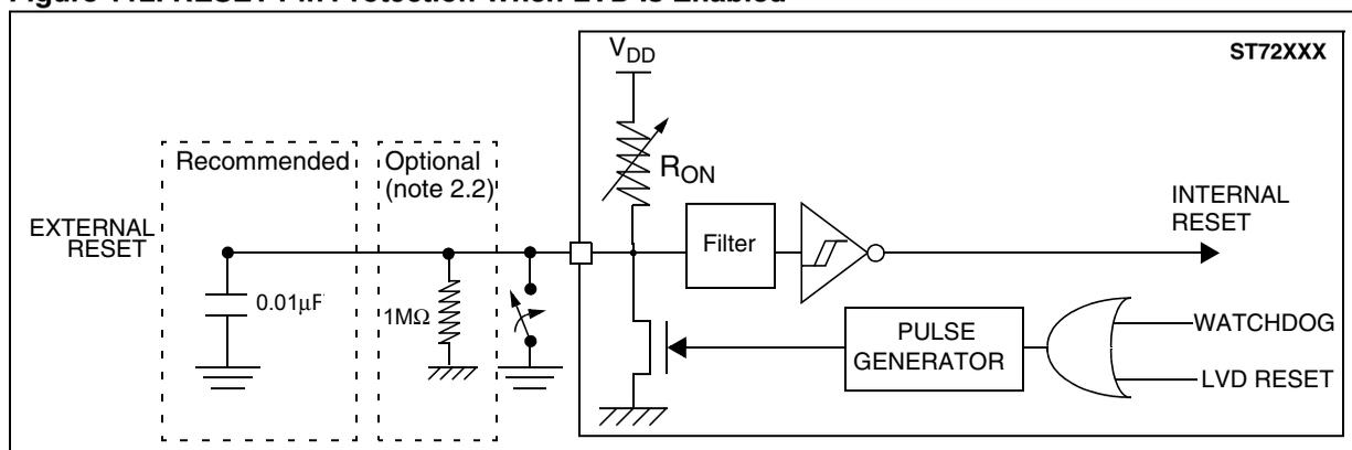
Figure 113.  $\overline{\text{RESET}}$  Pin Protection When LVD Is Disabled<sup>1)</sup>
