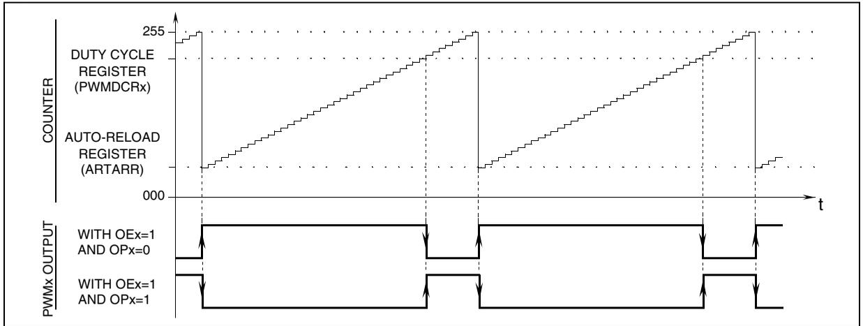
**Figure 43. PWM Signal from 0% to 100% Duty Cycle**
