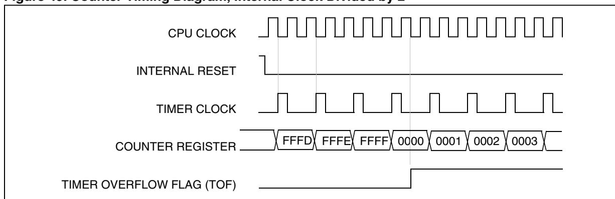
Figure 50. Counter Timing Diagram, Internal Clock Divided by 4
