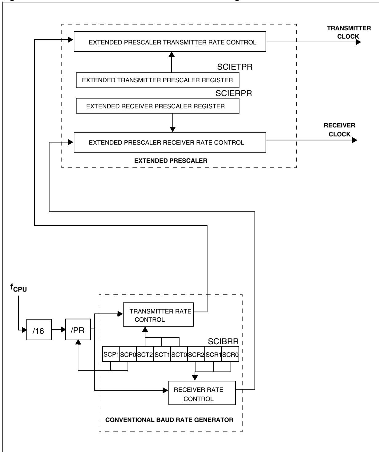
**LINSCI™ SERIAL COMMUNICATION INTERFACE (LIN Master Only) (Cont'd)****10.8.4.4 Conventional Baud Rate Generation**
