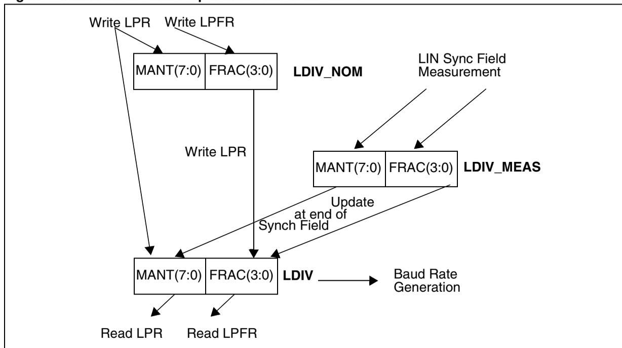
Figure 85. LDIV Read / Write Operations When LDUM = 1
