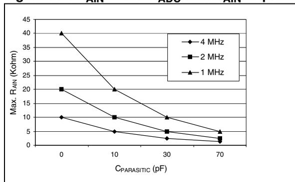
Figure 120. Recommended  $C_{AIN}/R_{AIN}$  Values<sup>3)</sup>
