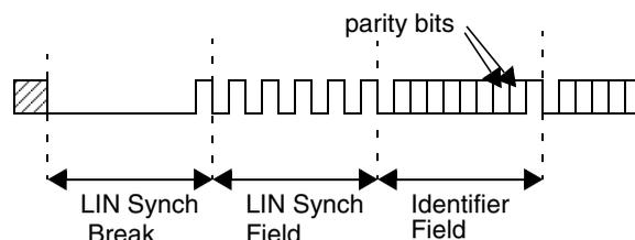
The bits involved are the two MSB positions (7th and 8th bits if M = 0; 8th and 9th bits if M = 0) of the identifier character. The check is performed as specified by the LIN specification:
