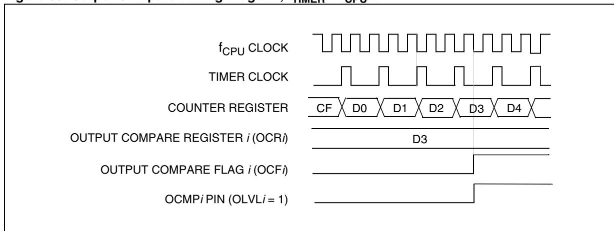
Figure 67. Output Compare Timing Diagram,  $f_{\text{TIMER}} = f_{\text{CPU}}/4$
