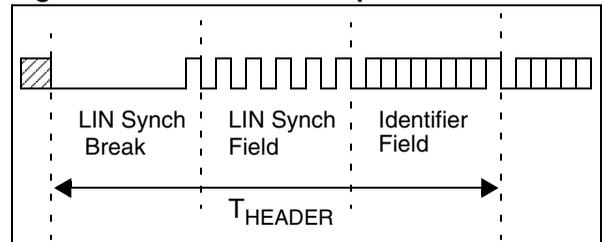
The time-out counter is enabled at each break detection. It is stopped in the following conditions:
