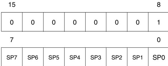
The Stack Pointer is a 16-bit register which is always pointing to the next free location in the stack. It is then decremented after data has been pushed onto the stack and incremented before data is popped from the stack (see Figure 2).
