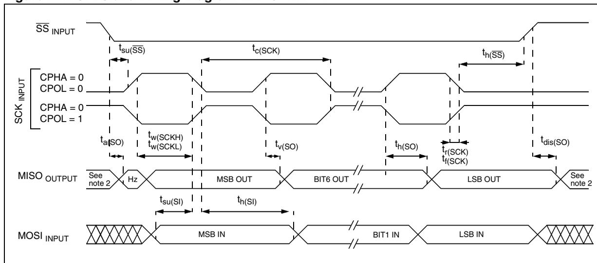
Figure 118. SPI Master Timing Diagram<sup>1)</sup>
