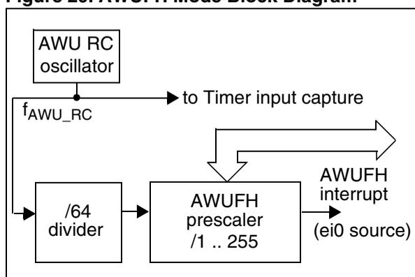
As soon as HALT mode is entered, and if the AWUEN bit has been set in the AWUCSR register, the AWU RC oscillator provides a clock signal ( $f_{AWU\_RC}$ ). Its frequency is divided by a fixed divider and a programmable prescaler controlled by the AWUPR register. The output of this prescaler provides the delay time. When the delay has elapsed the AWUF flag is set by hardware and an interrupt wakes up the MCU from Halt mode. At the same time the main oscillator is immediately turned on
