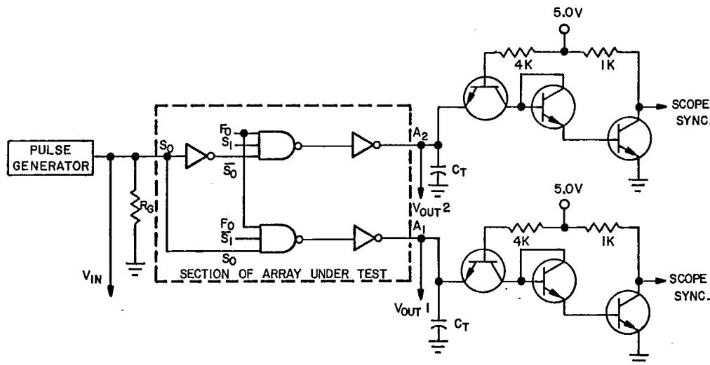
Illustrating a two-gate path from a control input to one output and a three-gate path from the same control input to another output. When  $\bar{S}_1 F_0 = 1$ , output  $A_1$  follows the input and appears after two gate delays. When  $\bar{S}_1 F_0 = 1$ , output  $A_2$  is the inverse of the input and appears after three gate delays.
