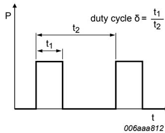
Fig. 17. Duty cycle definition
