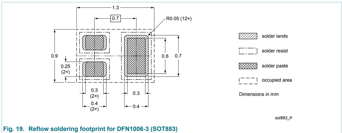
Fig. 19. Reflow soldering footprint for DFN1006-3 (SOT883)
