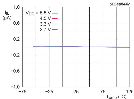
Fig 19. LOW-level input current versus temperature; digital pins
