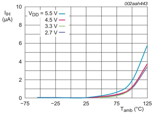
**Fig 20. HIGH-level input current versus temperature; digital pins**
