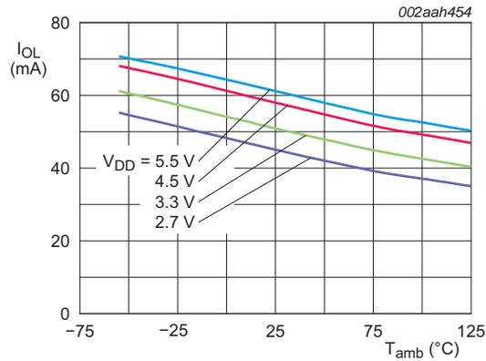
**Fig 22. LOW-level output current on SDA pin versus temperature; V<sub>OL</sub> = 0.4 V**
