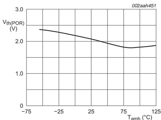
**Fig 24. Power-on reset threshold voltage versus temperature; rising V<sub>CC</sub>**
