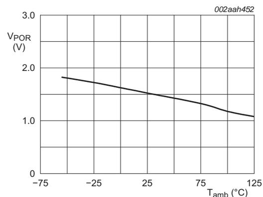
**Fig 25. Power-on reset voltage versus temperature; falling V<sub>CC</sub>**
