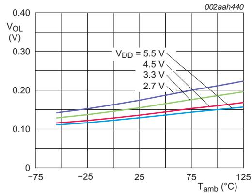
Fig 17. LOW-level output voltage on OS pin versus temperature; I<sub>OL</sub> = 4 mA
