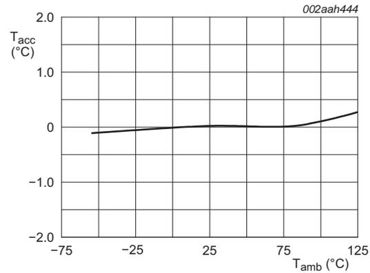
**Fig 23. Temperature accuracy versus temperature; V<sub>CC</sub> = 2.8 V to 5.5 V**
