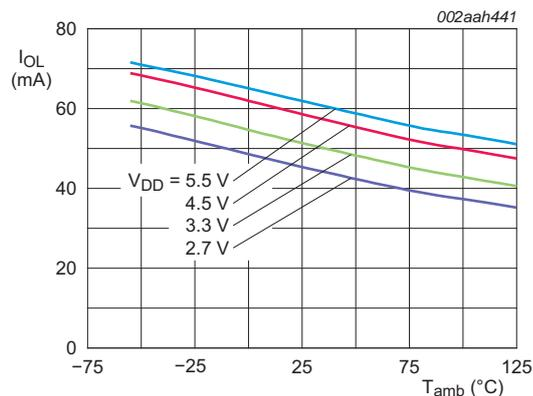
Fig 18. LOW-level output current on OS pin versus temperature; V<sub>OL</sub> = 0.4 V
