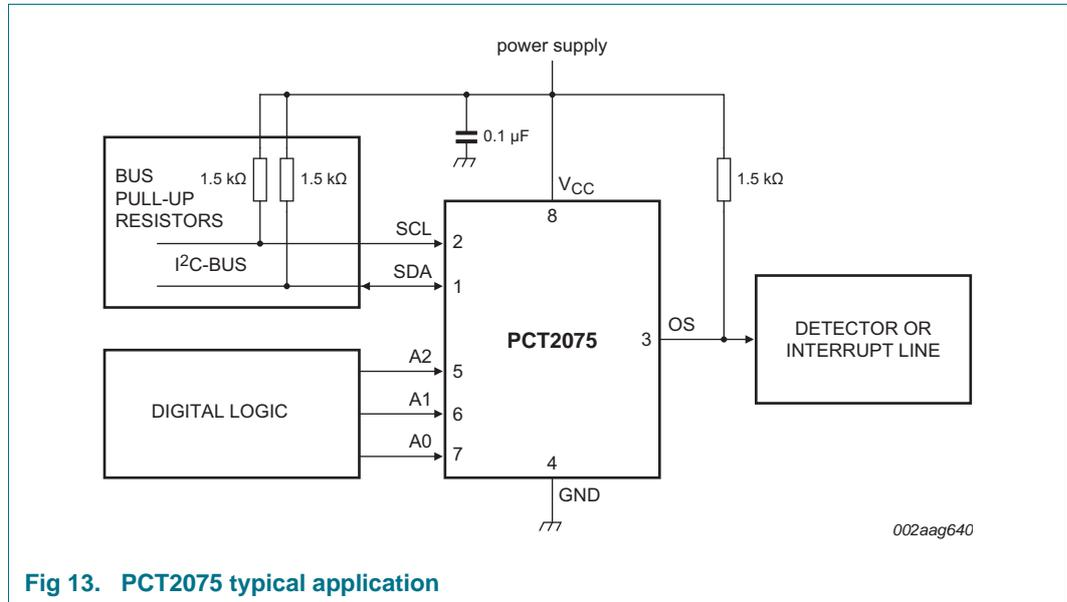
Fig 13. PCT2075 typical application
