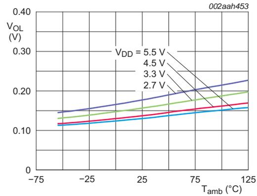
**Fig 21. LOW-level output voltage on SDA pin versus temperature; I<sub>OL</sub> = 20 mA**
