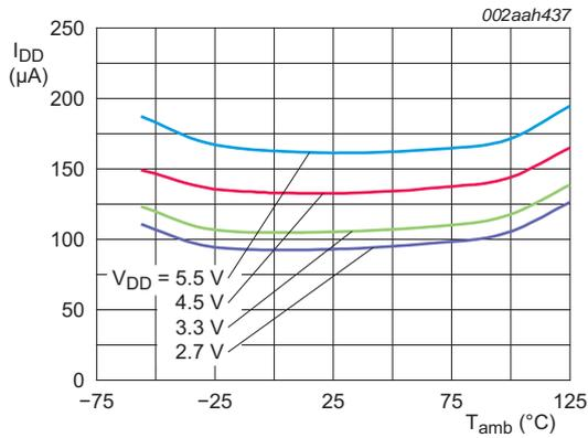
Fig 14. Average supply current versus temperature; I<sup>2</sup>C-bus inactive
