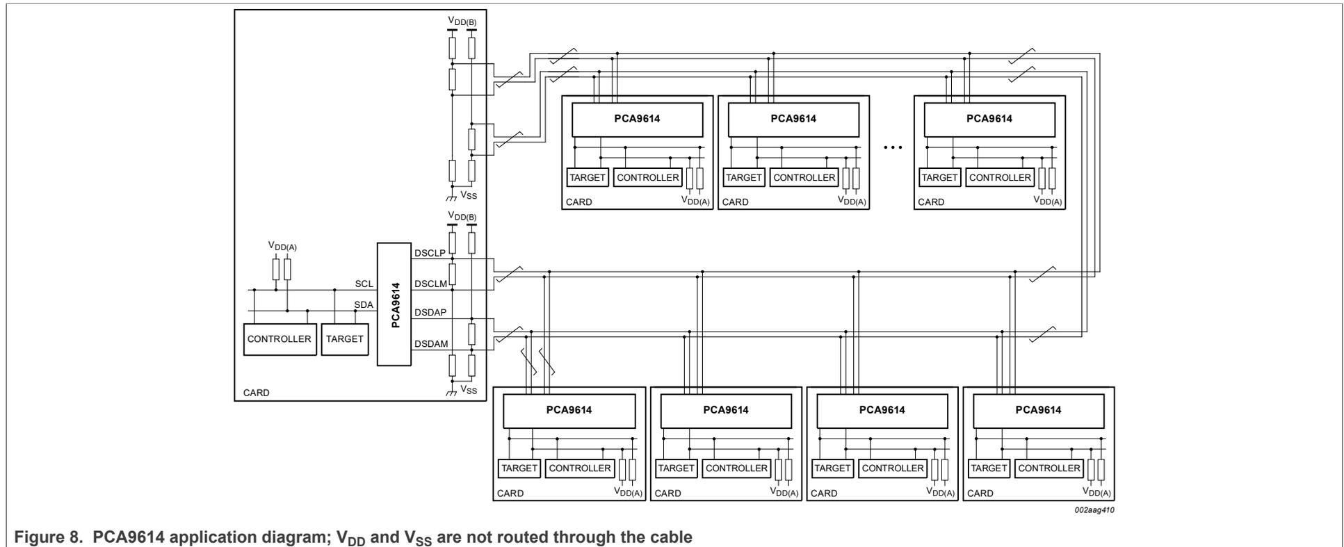
Figure 8. PCA9614 application diagram; V<sub>DD</sub> and V<sub>SS</sub> are not routed through the cable
