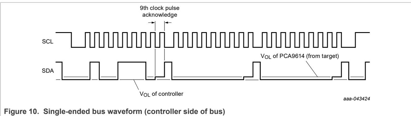
Figure 10. Single-ended bus waveform (controller side of bus)
