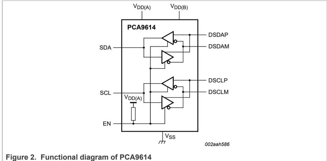
Figure 2. Functional diagram of PCA9614
