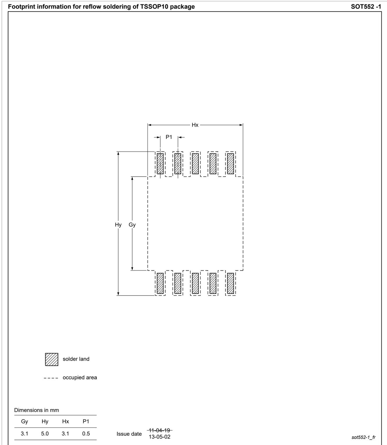
Figure 18. PCB footprint for SOT552-1 (TSSOP10); reflow soldering
