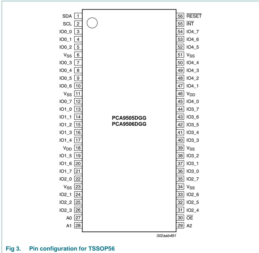
Fig 3. Pin configuration for TSSOP56
