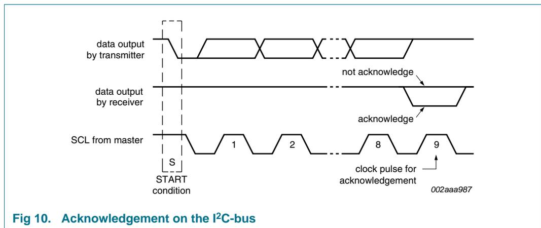
Fig 10. Acknowledgement on the I<sup>2</sup>C-bus
