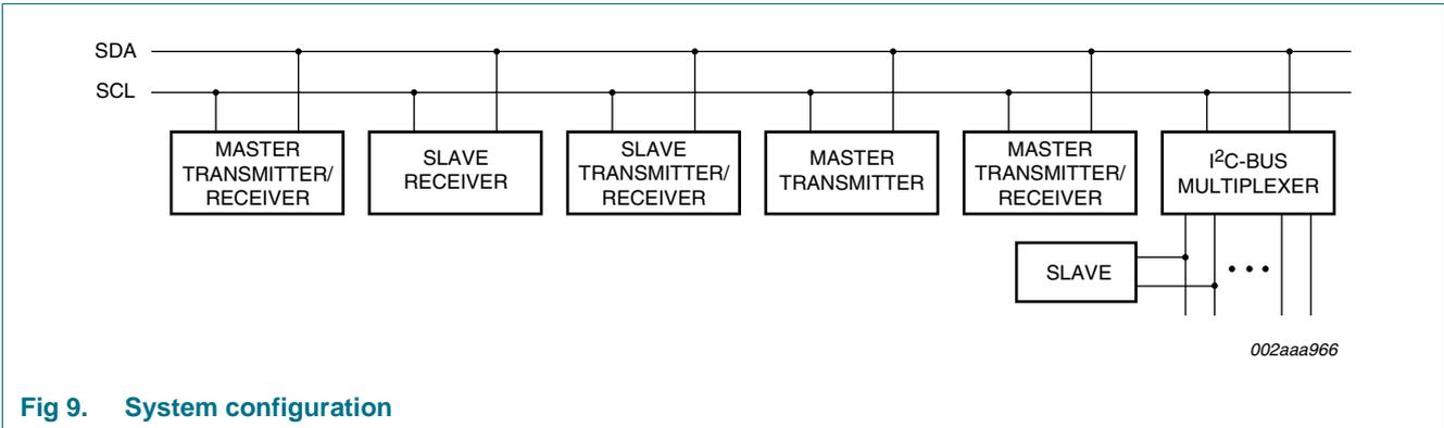
Fig 9. System configuration
