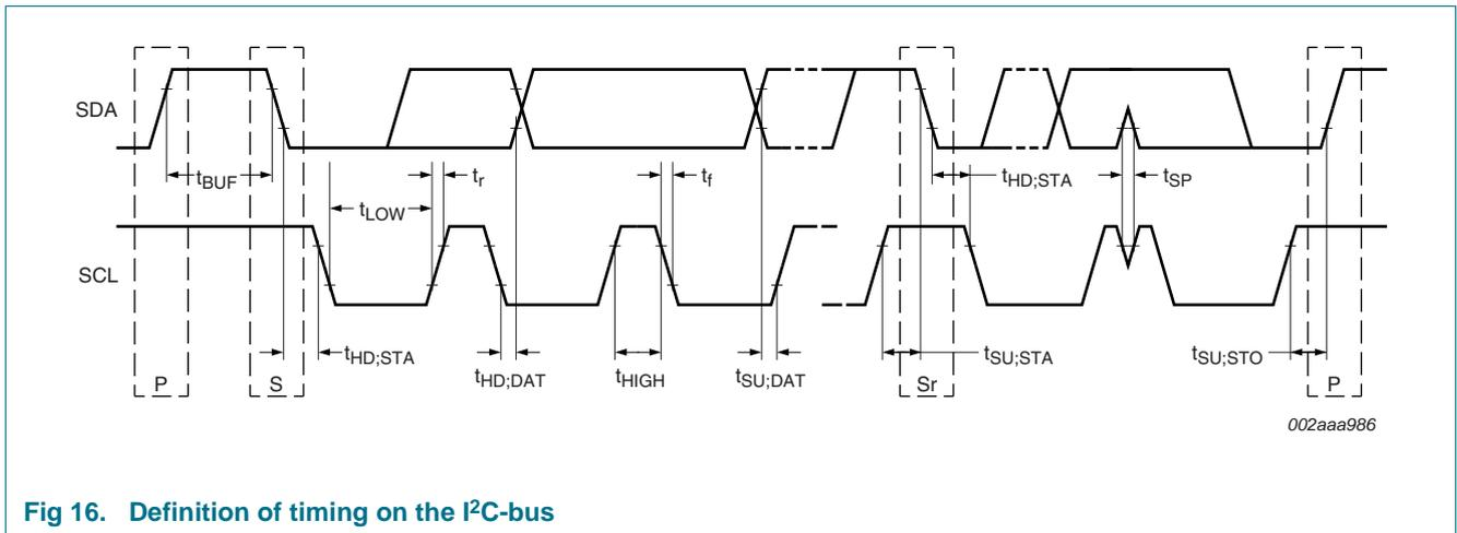
Fig 16. Definition of timing on the I<sup>2</sup>C-bus
