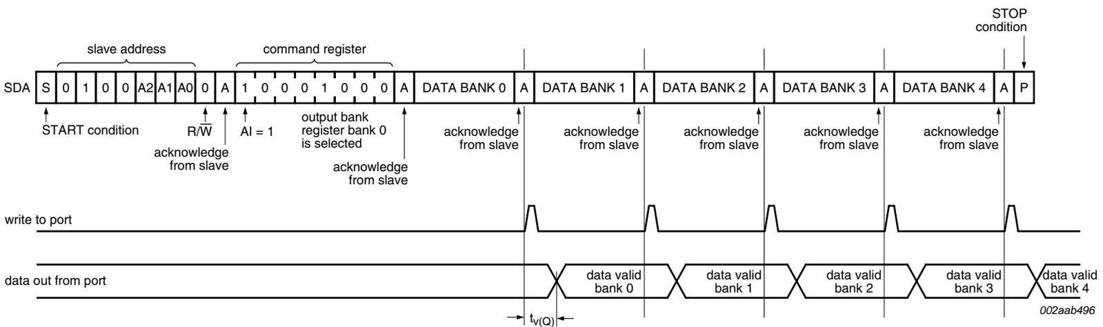
$\overline{\text{OE}}$  is LOW to observe a change in the outputs.
