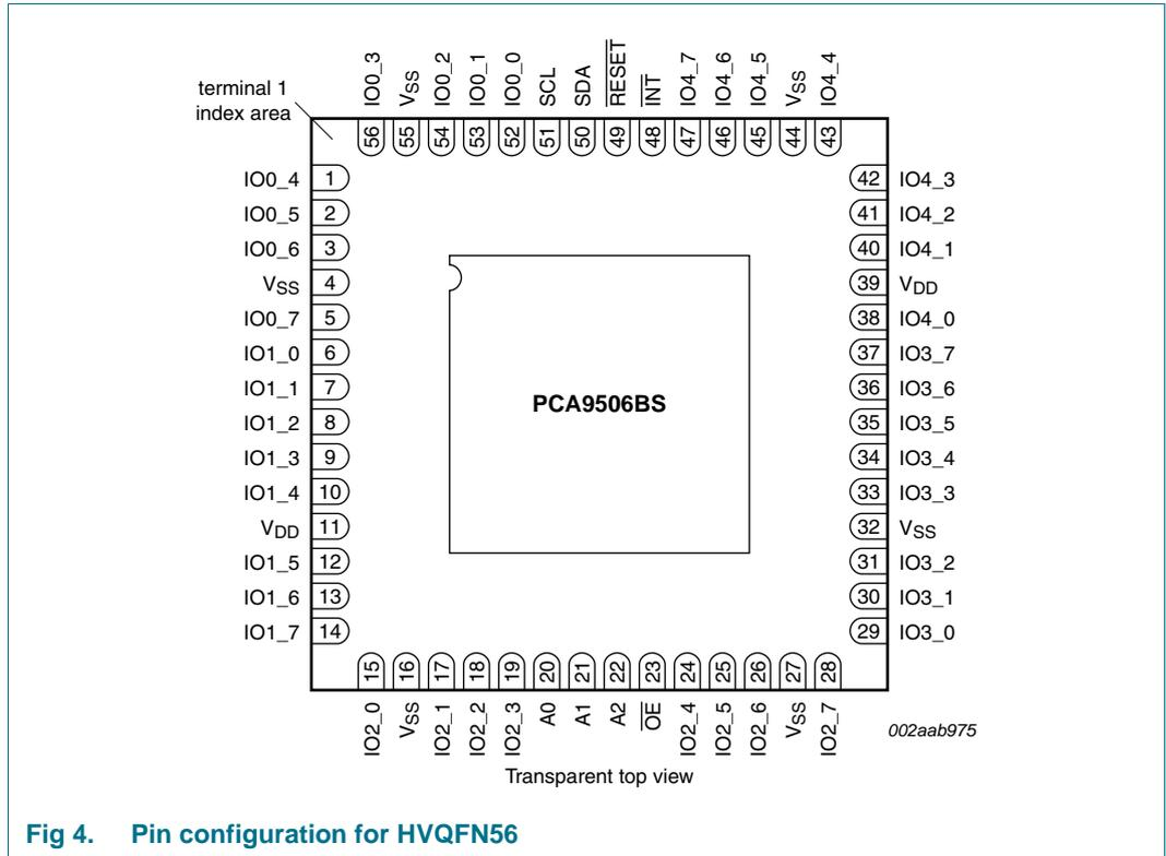
Fig 4. Pin configuration for HVQFN56
