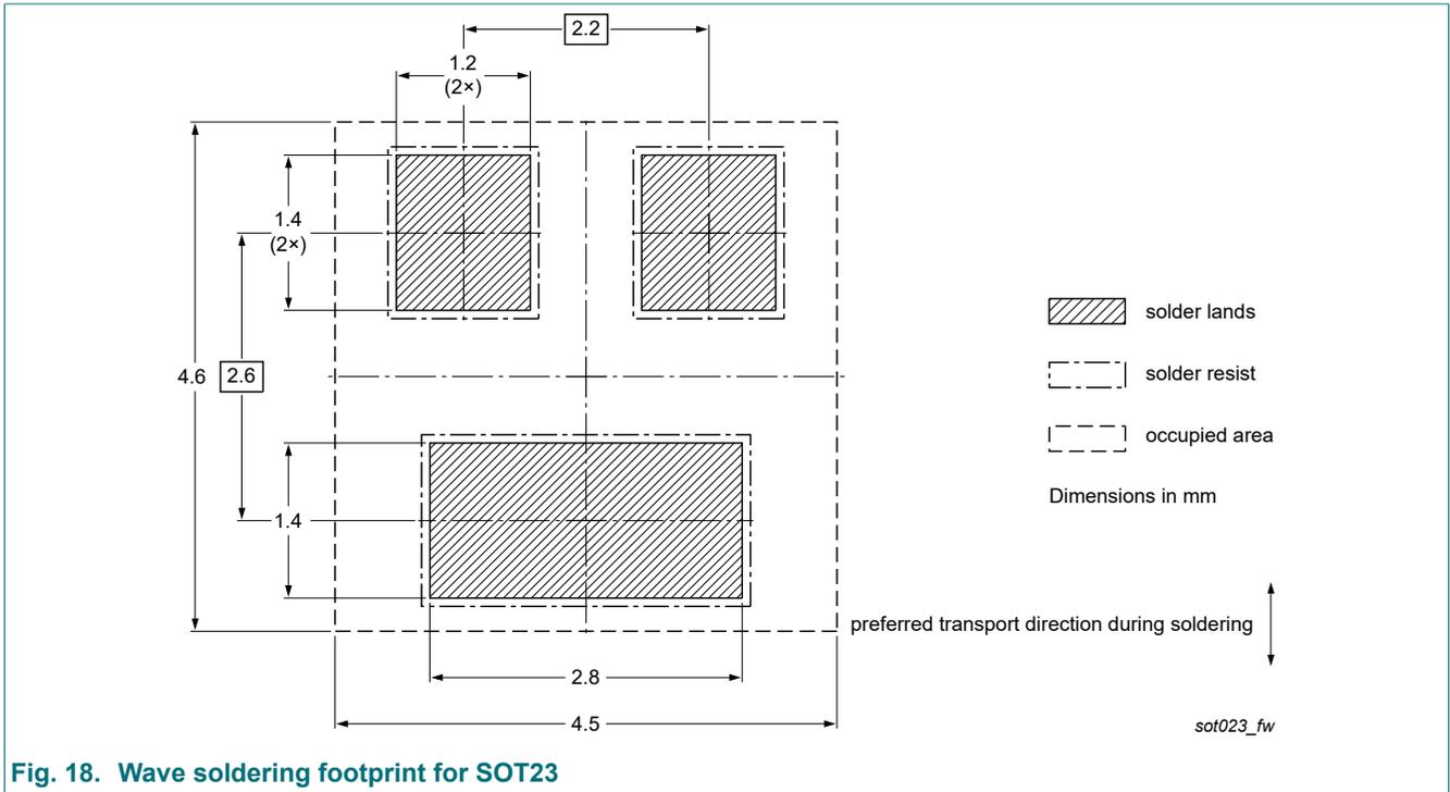
Fig. 18. Wave soldering footprint for SOT23
