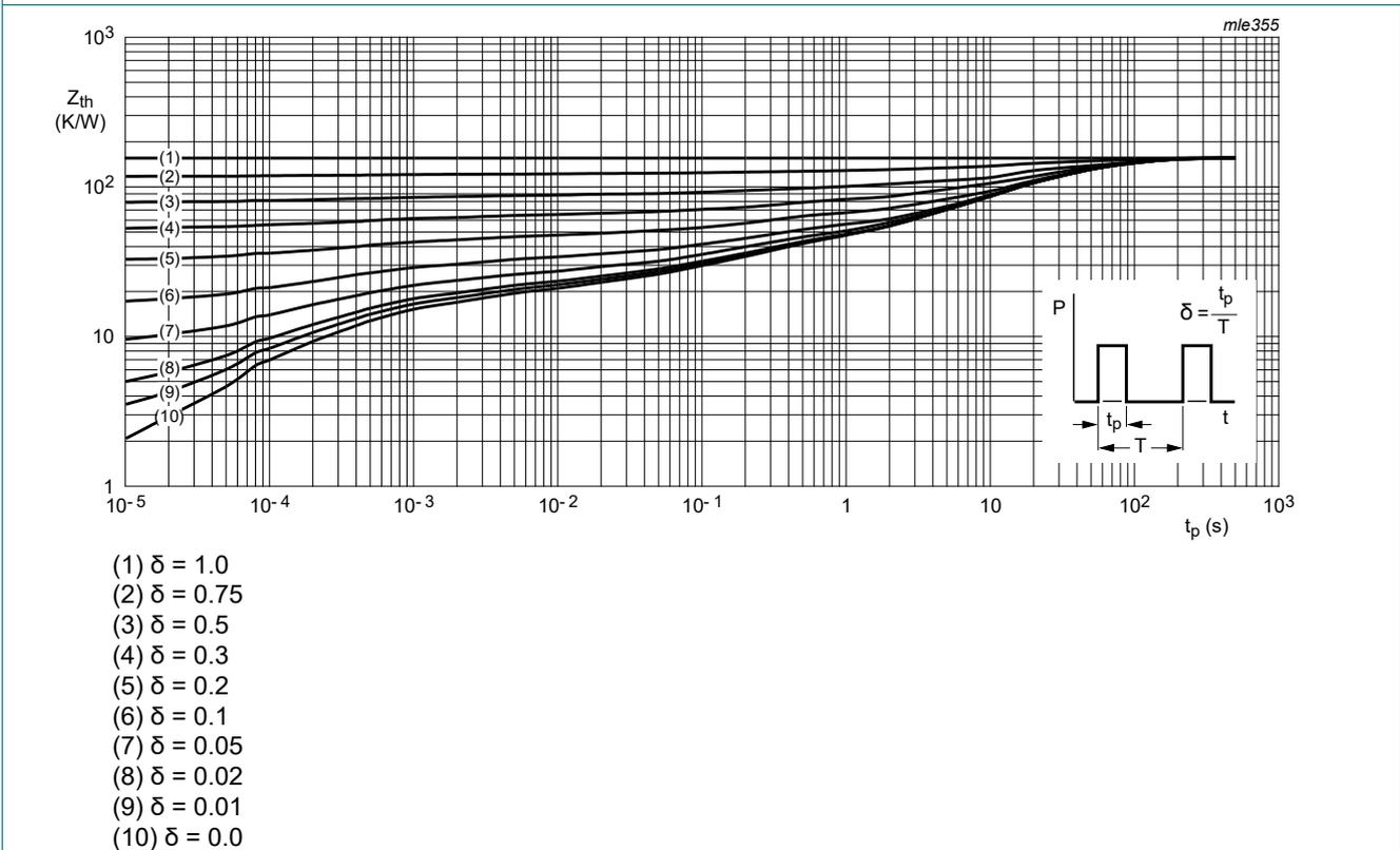
**Fig. 3. Transient thermal impedance as a function of pulse time for collector 1 cm<sup>2</sup> copper mounting pad**
