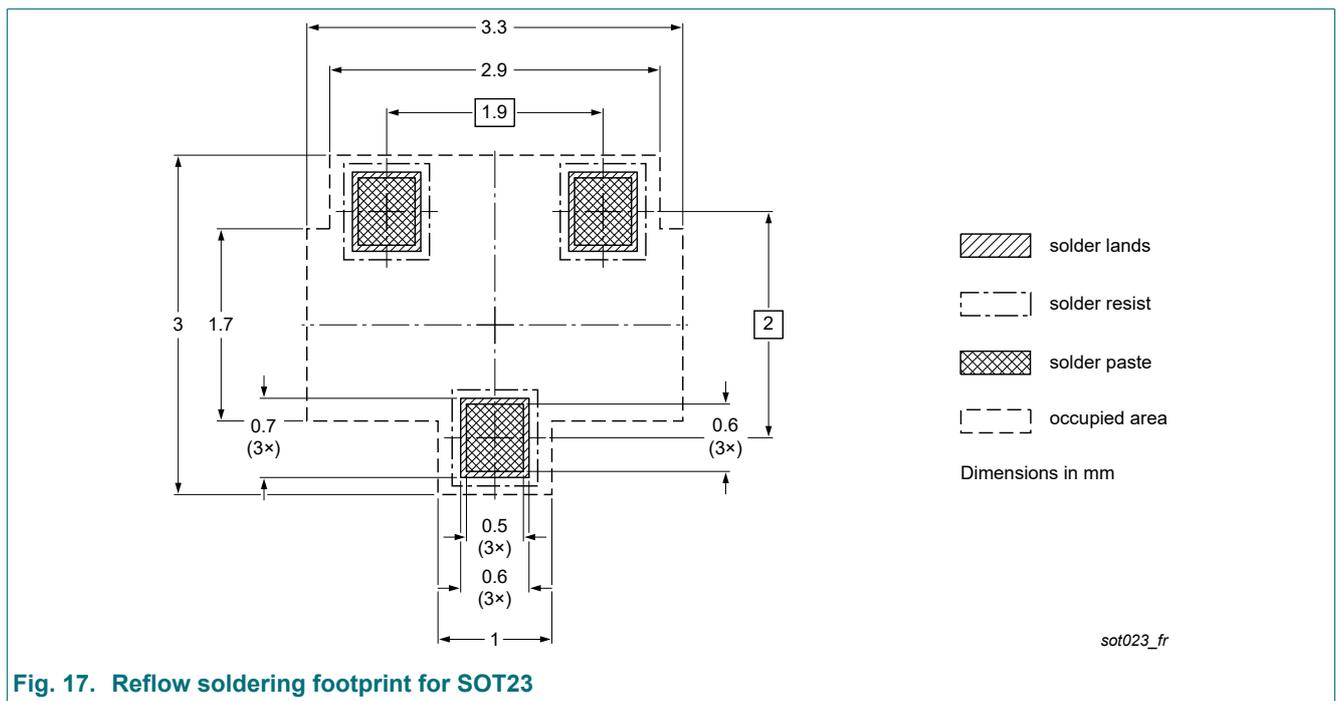
Fig. 17. Reflow soldering footprint for SOT23
