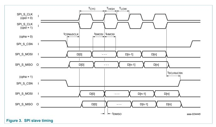
Write operations of NXH3670UK SPI slave interface can be done with a clock frequency of 16 MHz. However, for read operations in the final application, the MISO output delay can impact the performances.
