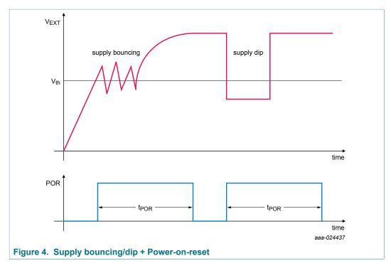
When  $V_{EXT}$  drops below  $V_{POR}$ , the power-on reset circuit drives the RESETN signal LOW weakly to generate a clean reset signal to reset the PMU. The PMU prolongs the reset for  $t_{POR}$  to reset the rest of the chip. When not active, the power-on reset circuit is driving the RESETN signal weakly HIGH (see Figure 5).
