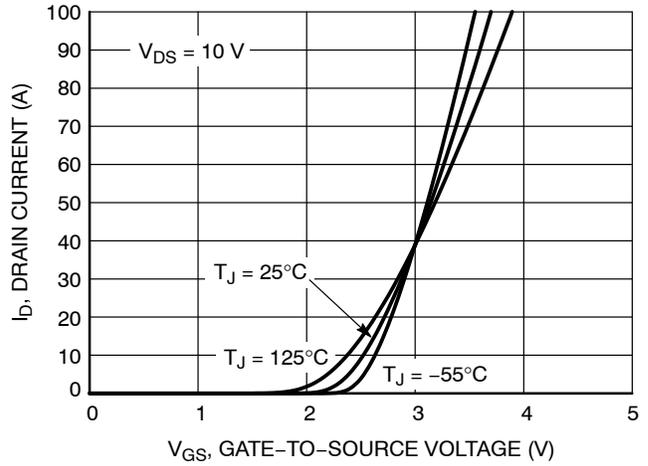
Figure 2. Transfer Characteristics
