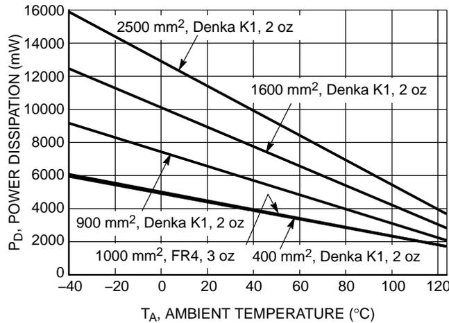
Figure 6. Power Dissipation vs. Ambient Temperature @  $T_J = 175^\circ\text{C}$
