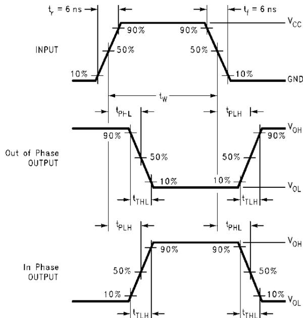
Figure 6. AC Waveforms
