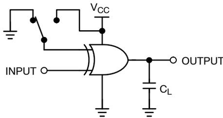
C<sub>L</sub> includes load and stray capacitance
