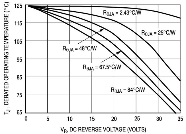
Figure 8. Typical Operating Temperature Derating Per Leg \*
