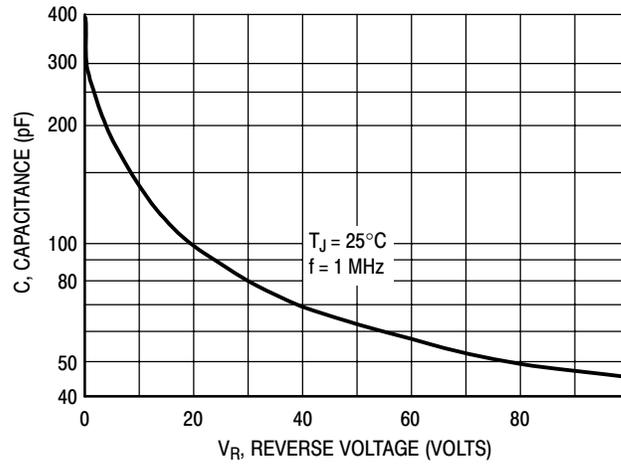
**Figure 5. Typical Capacitance**
