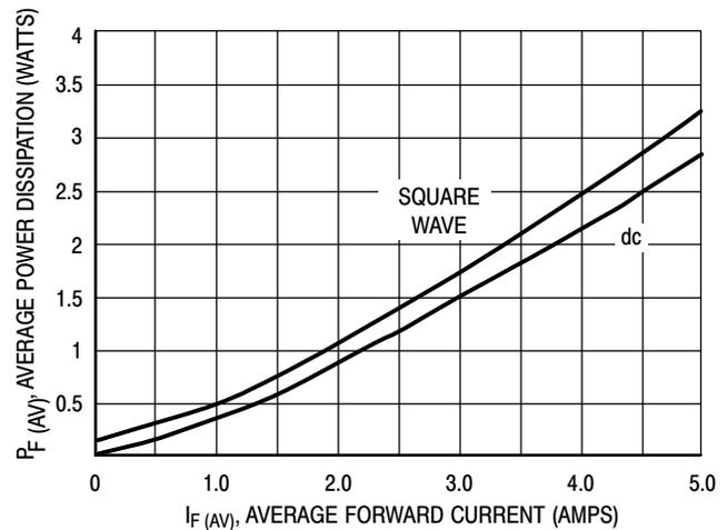
Figure 4. Power Dissipation
