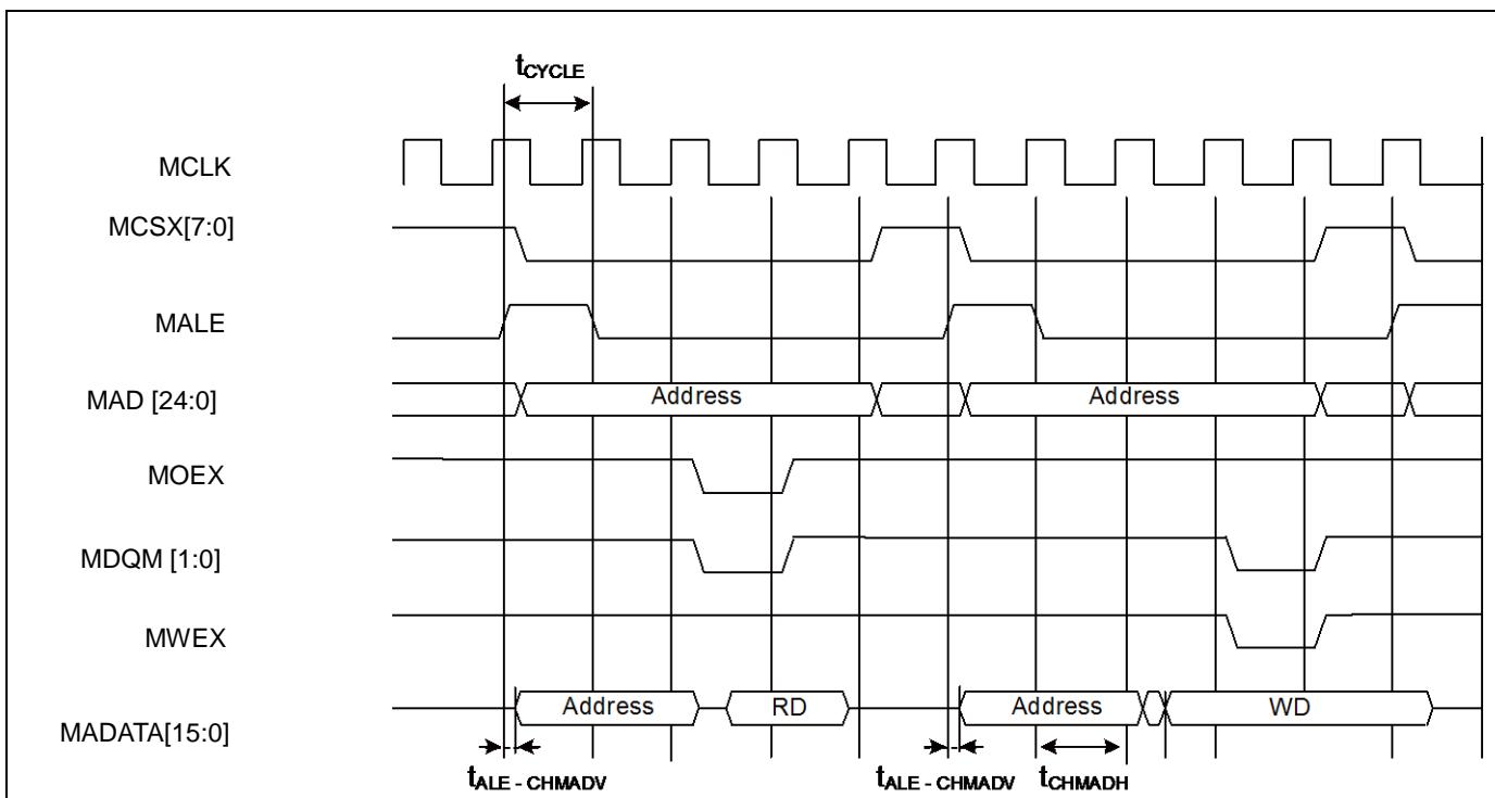
**Multiplexed Bus Access Synchronous SRAM Mode**
