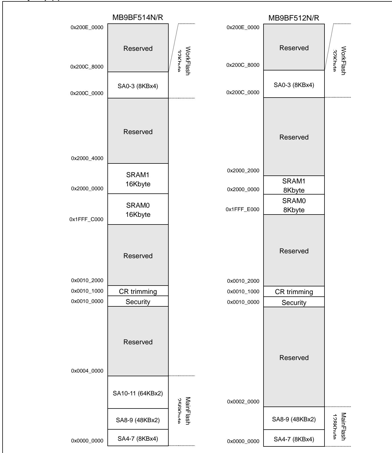
See "MB9B510R/410R/310R/110R Series Flash programming Manual" for sector structure of Flash.
