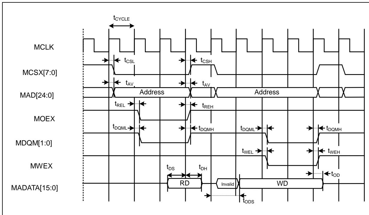
**Multiplexed Bus Access Asynchronous SRAM Mode**
