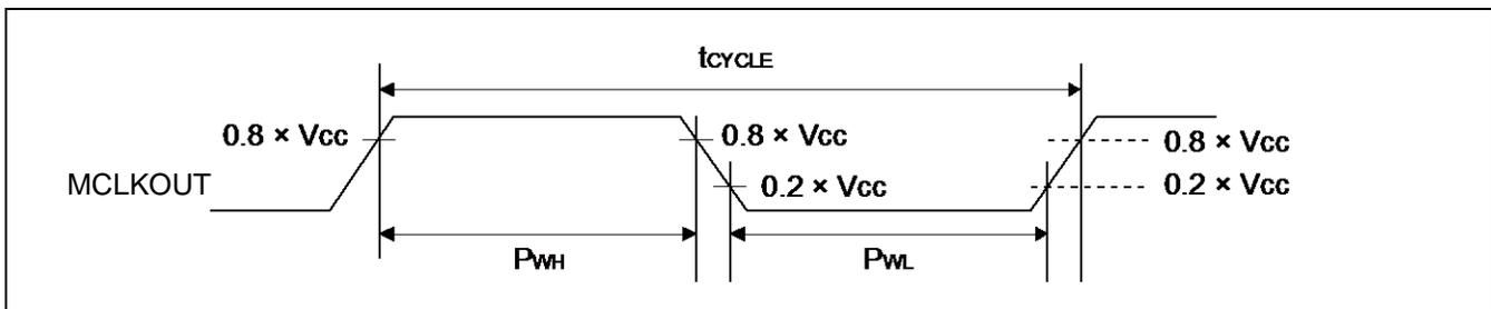
**External bus signal input/output Characteristics**
