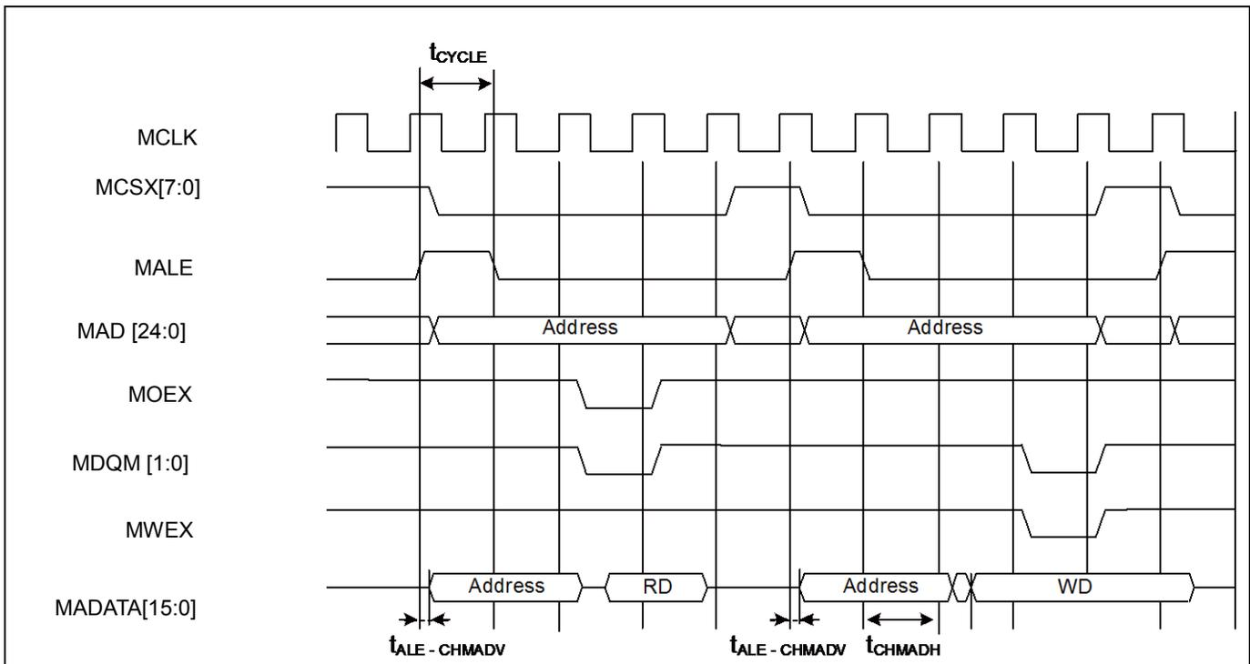
**Multiplexed Bus Access Synchronous SRAM Mode**
