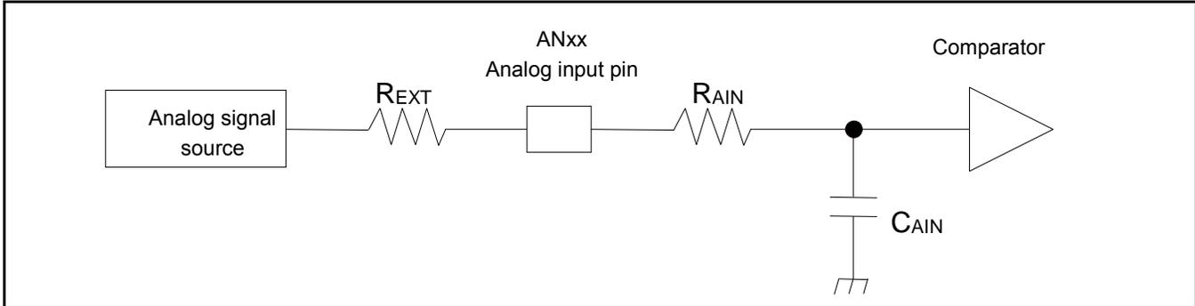
(Equation 1)  $t_s \geq (R_{AIN} + R_{EXT}) \times C_{AIN} \times 9$
