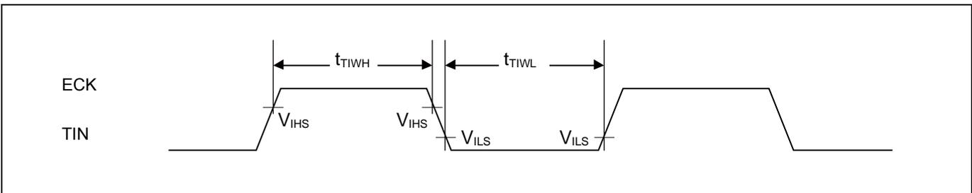
**Trigger input timing**
