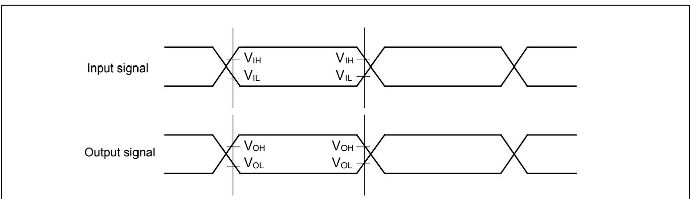
**Separate Bus Access Asynchronous SRAM Mode**
