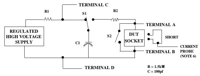
other input and output pins connected to terminal B. All pins except the input or output pin being tested and the Mil Std 883D combination of all the other input and output pins shall be open.
