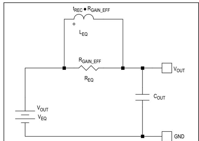
Figure 4. Averaged Small-Signal Equivalent Circuit of Regulator
