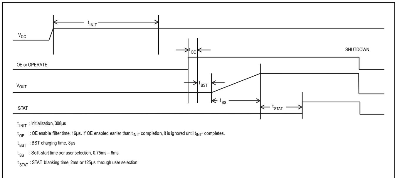
Figure 1. Startup Timing
