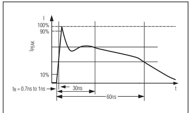
Figure 3d. IEC 61000-4-2 ESD Generator Current Waveform
