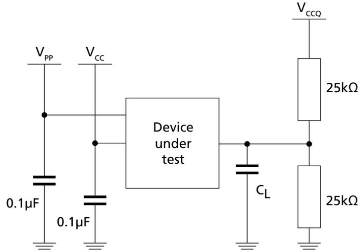
Note: 1.  $C_L$  includes jig capacitance.
