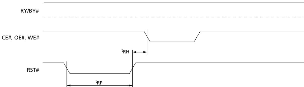
**Figure 14: Reset AC Timing During PROGRAM/ERASE Operation**
