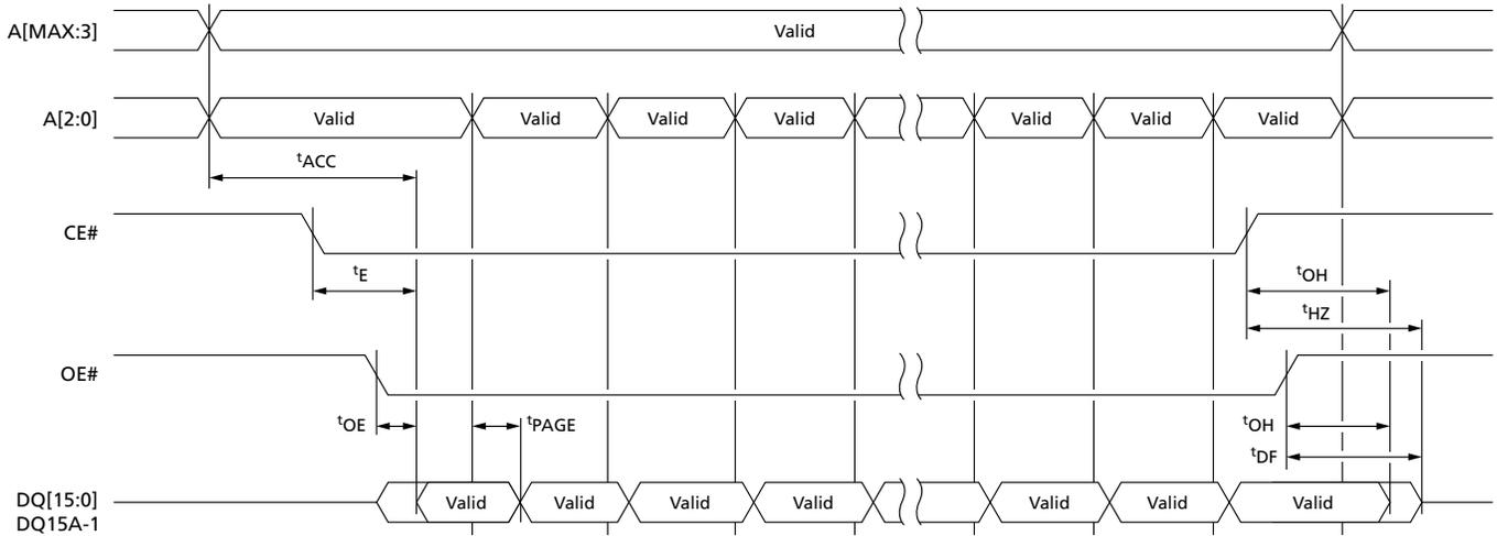
Note: 1. Page size is 8 words (16 bytes) and is addressed by address inputs A[2:0] in x16 bus mode and A[2:0] plus DQ15/A-1 in x8 bus mode.
