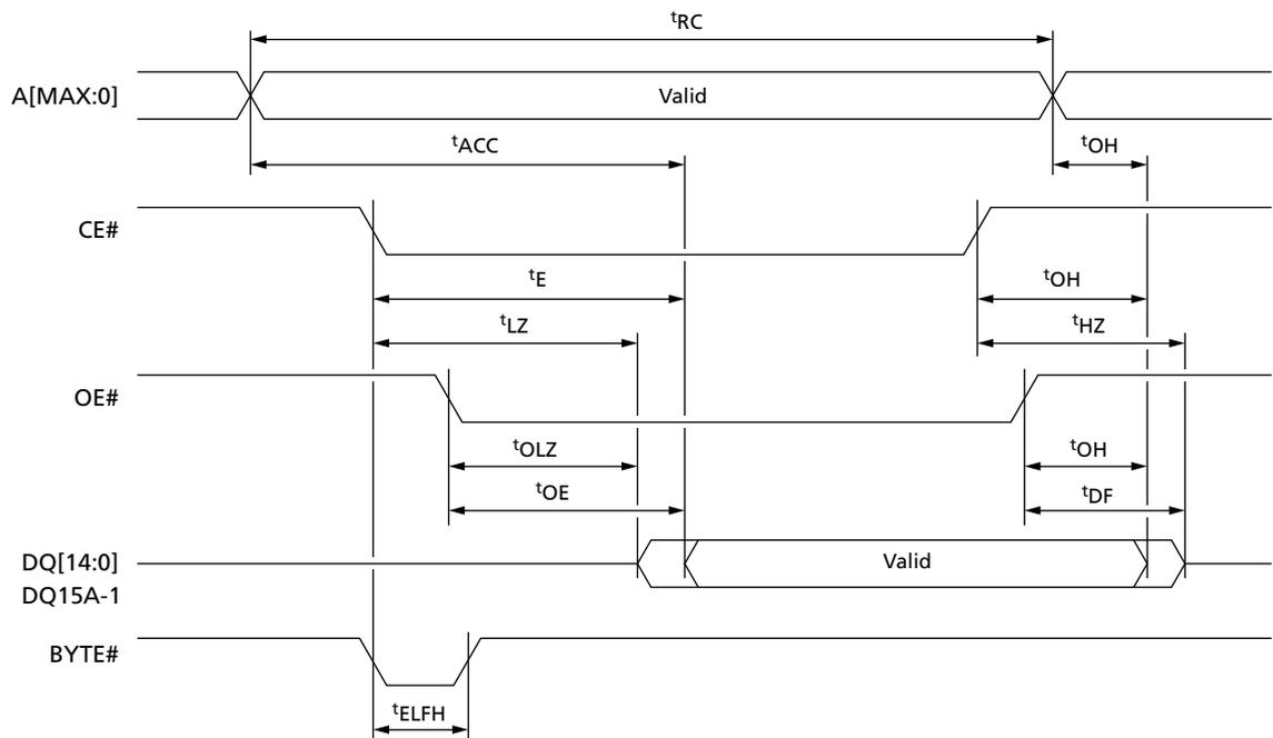
**Figure 19: Page Read AC Timing (16-Bit Mode)**
