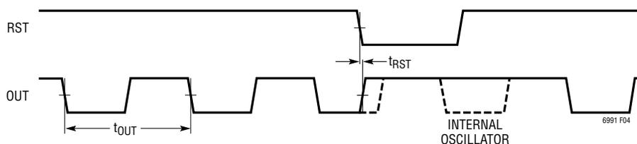
**Figure 4. RST Timing Diagram (POL = 1)**
