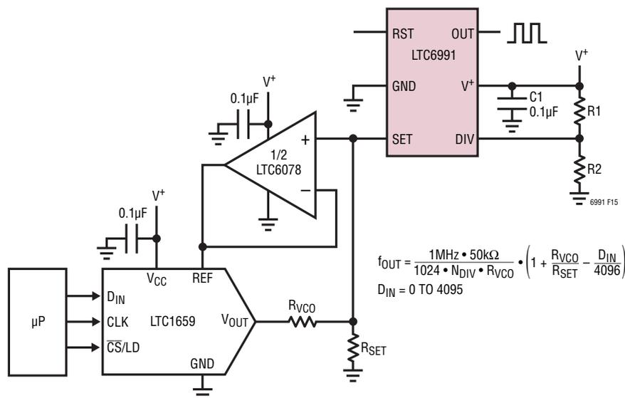
Figure 15. Digitally-Controlled Oscillator
