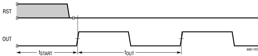
Figure 7. Start-Up Timing Diagram (RST = 0, POL = 0)
