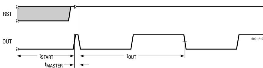
Figure 10. Start-Up Timing Diagram (RST = 1, POL = 1)
