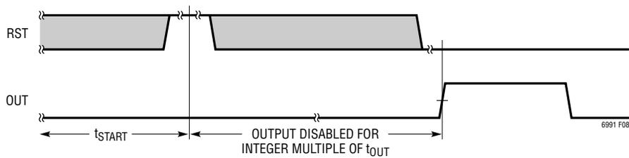
Figure 8. Start-Up Timing Diagram (RST = 1, POL = 0)
