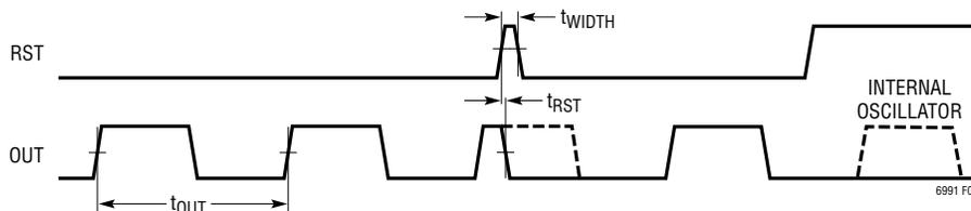
**Figure 3. RST Timing Diagram (POL = 0)**
