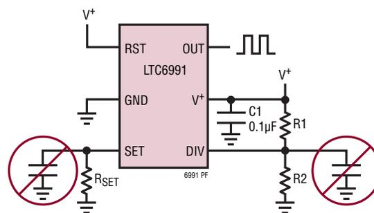
**RST (Pin 4/Pin 1):** Output Reset. The behavior of the RST pin is dependent on the polarity bit (POL). The POL bit is configured via the DIVCODE setting. When POL = 0, setting RST high forces OUT low and setting RST low allows the output to oscillate. When POL = 1, RST is active low. In that case, setting RST low forces OUT high and setting RST high allows the output to oscillate.
