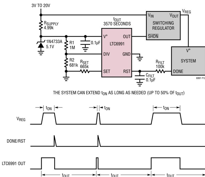
Figure 12. Powering Up a System Once an Hour
