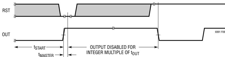
Figure 9. Start-Up Timing Diagram (RST = 0, POL = 1)
