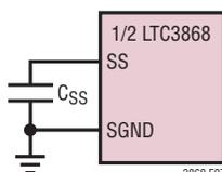
Figure 7. Using the TRACK/SS Pin to Program Soft-Start
