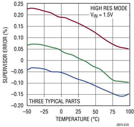
**Current Supervisor Total Unadjusted Error vs Temperature**
