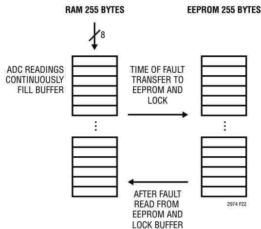
Figure 22: Fault Logging
