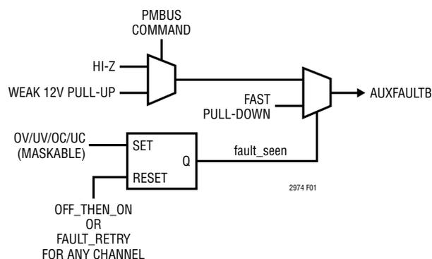
Figure 1: AUXFAULTB MUX
