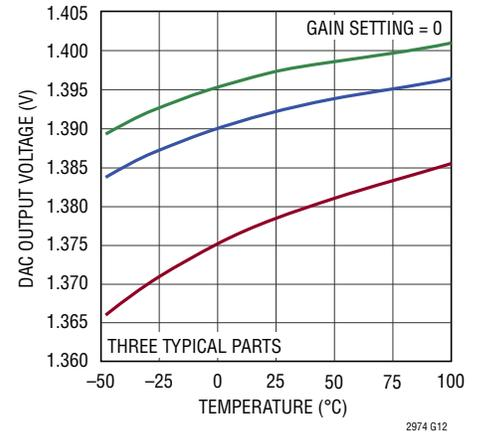
**DAC Full-Scale Voltage vs Temperature, Gain = 1**
