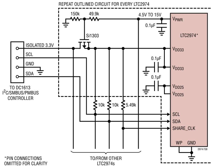
Figure 38. DC1613 Controller Connections When V<sub>PWR</sub> Is Used
