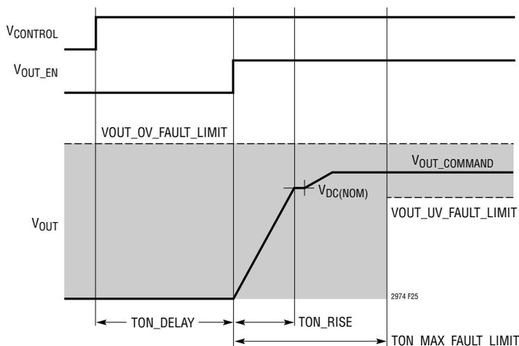
Figure 25. Typical ON Sequence Using Control Pin
