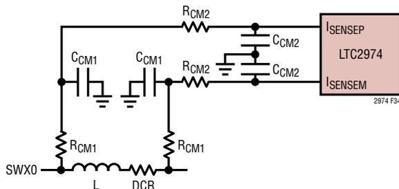
Figure 34. DCR Current Sensing Circuits
