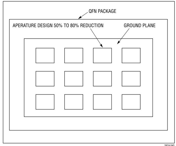
Figure 42. Suggested Screen Pattern for Die Attach Pad
