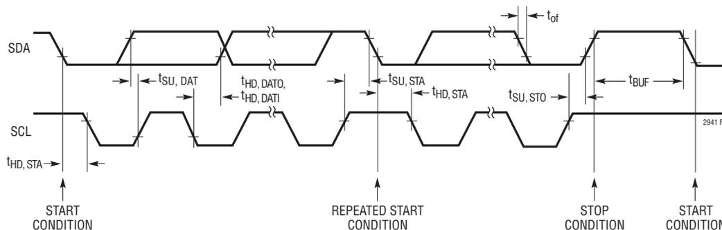
Figure 1. Definition of Timing on I<sup>2</sup>C Bus
