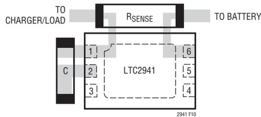
Figure 10. Kelvin Connection on Sense Resistor
